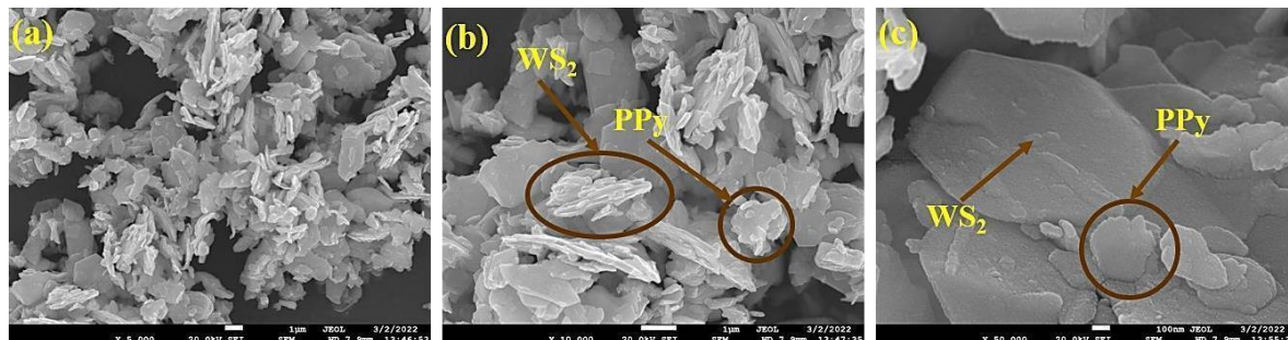
Figure 4.11 FE-SEM images of (a) Pure WS 2 (b) PPy/WS 2 - 5 wt% (10,000X) (c) PPy/WS 2 - 30 wt% (50,000X).
