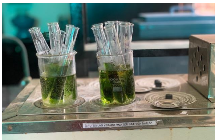
Figure 3.15 Leaf samples on the water bath for chlorophyll estimation
