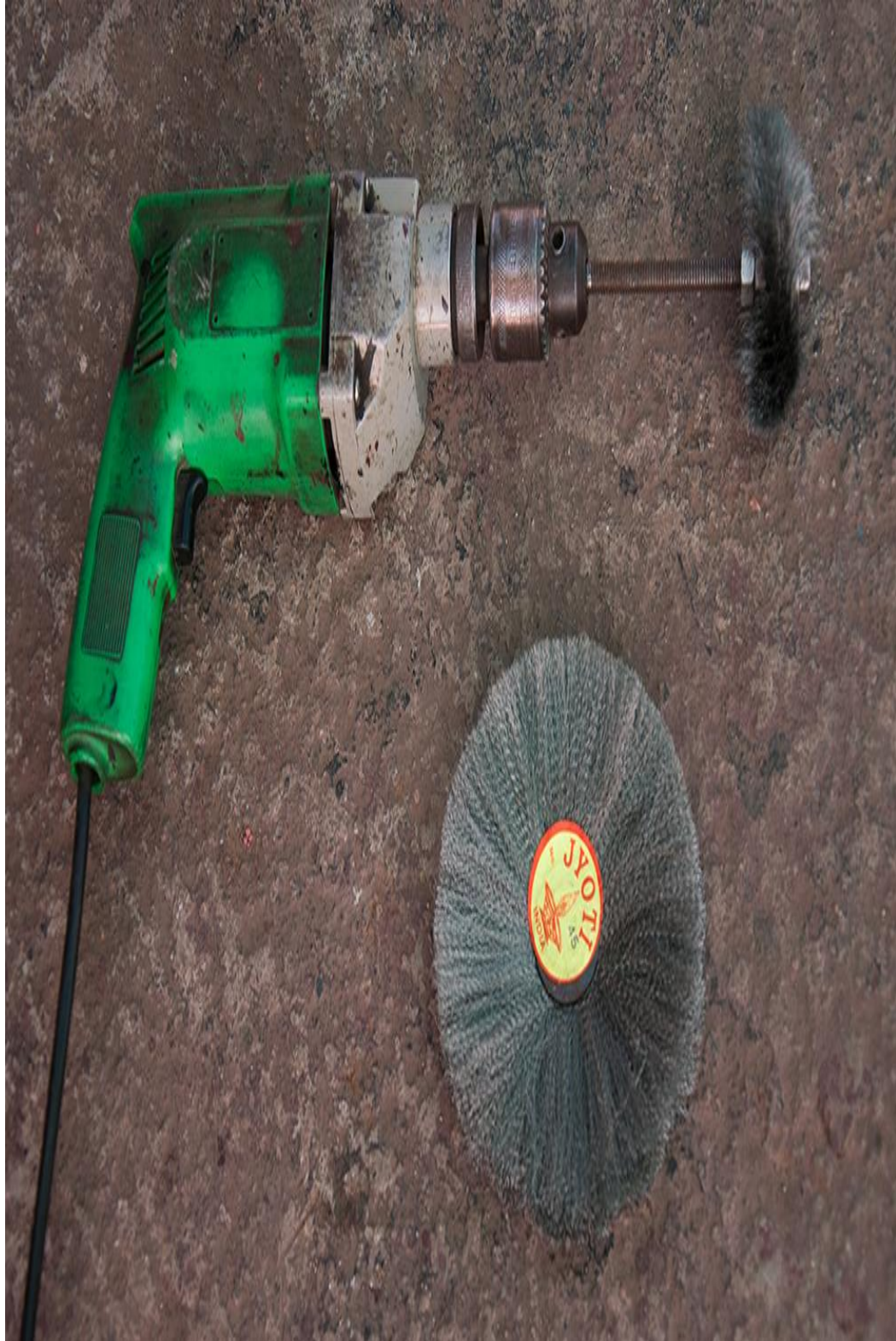
Figure 4.4: A buffing machine is used to smoothen the metal surfaces
