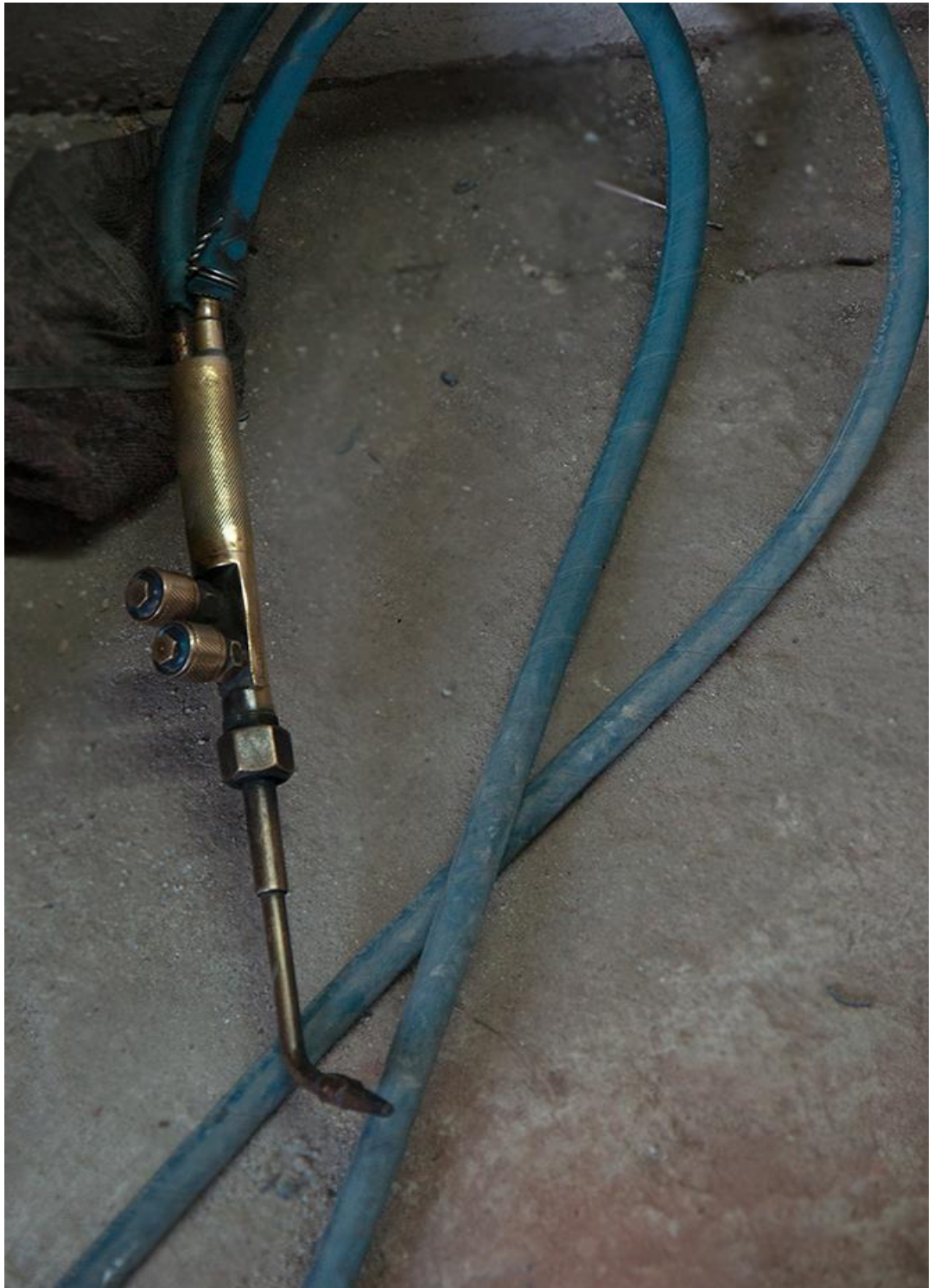
Figure 4.3: Gas welding torch connected to two gas hoses, one of the hoses realizes LPG while the other oxygen.
