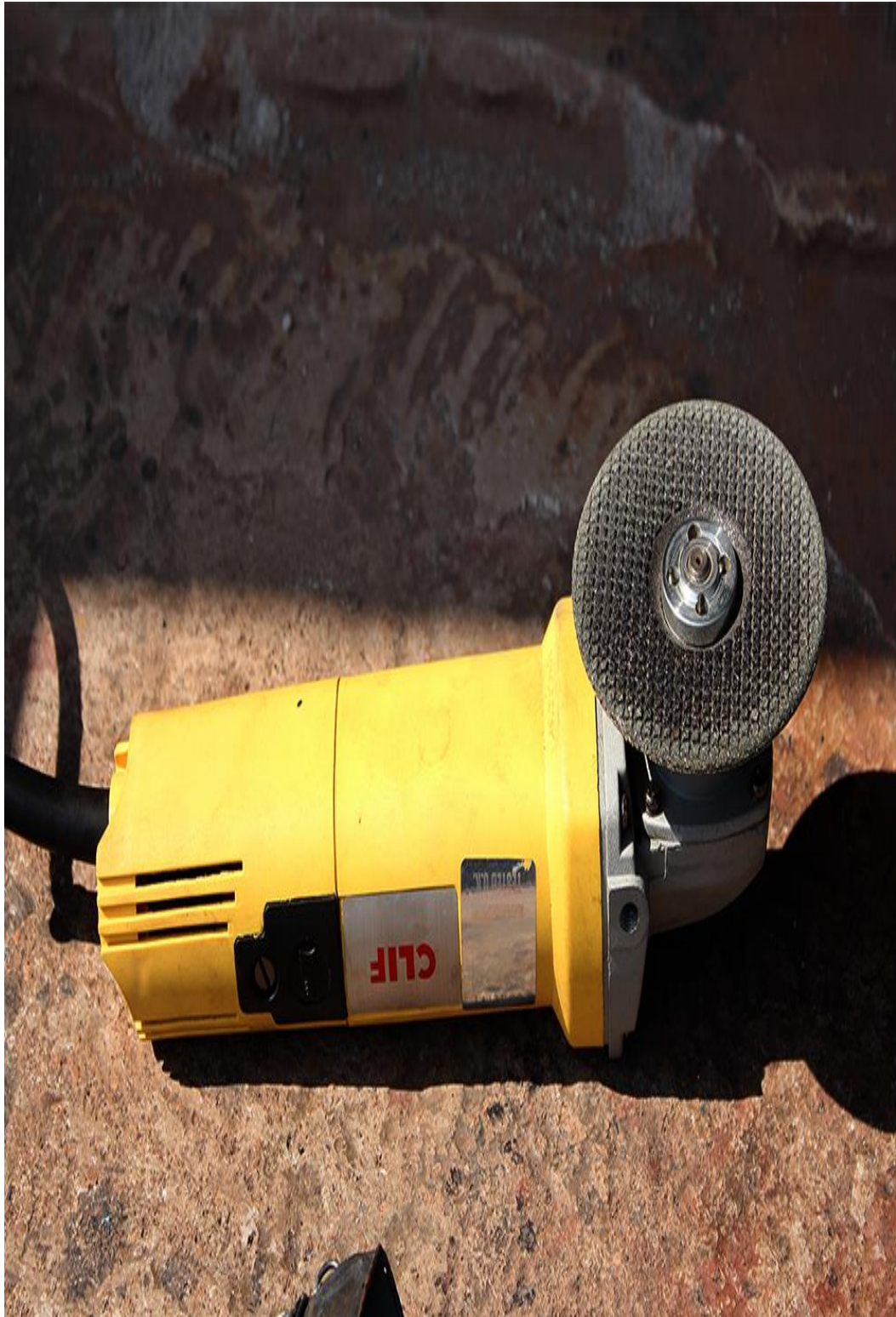
Figure 4.5: A grinding machine is used to remove excess pieces from the craft after welding.
