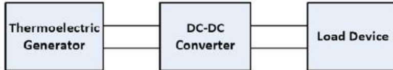
Figure:5.13 Simplified TEG system diagram
