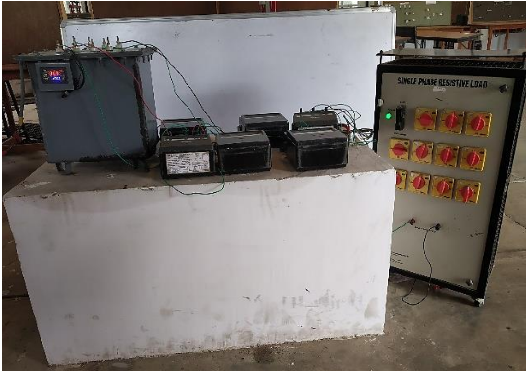
Fig.4.1(c) Experimental Setup showing Ester-Filled Transformer Connected to Single-Phase Resistive Load
