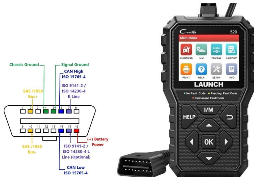
Fig.3.6. (a)OBD connector pinout, (b)OBD scanner
