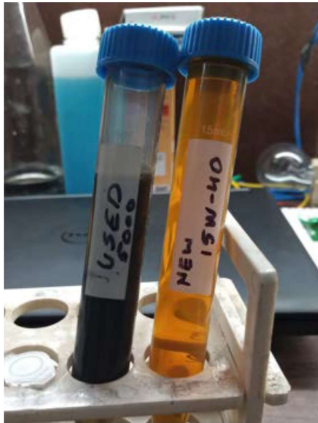
Fig. 4.1. Color relation of the sample left used and right unused engine oil The simplified structures represented in Fig.4.1 represent selected elements and functional entities, which may differ in execution from what is shown. The
