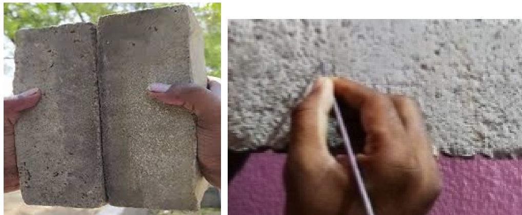
a) b) Figure 5.4 a) Soundness Test, b) Hardness Observation
