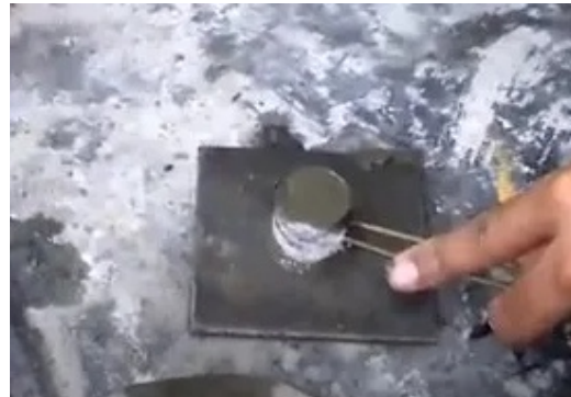
Figure 4.6 Le-Chatelier Apparatus to find Soundness of Cement
