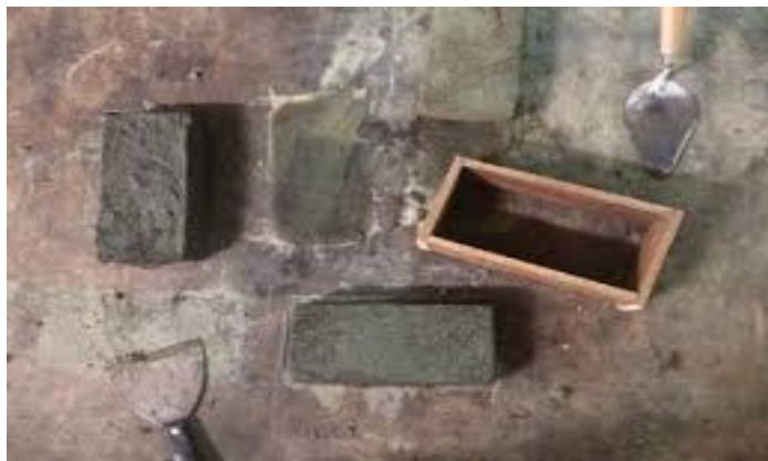
Figure 4.9 De-Moulding the Specimens
