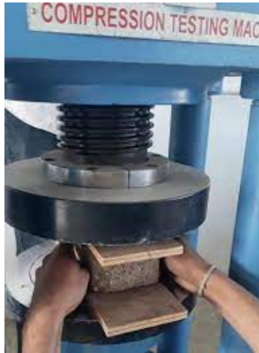
Figure 5.3 Compressive Strength Test of the Specimens
