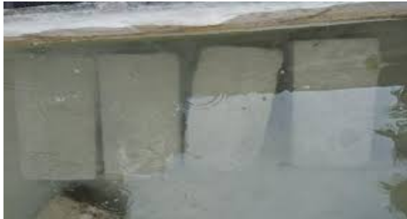
Figure 4.10 Curing of Specimens
