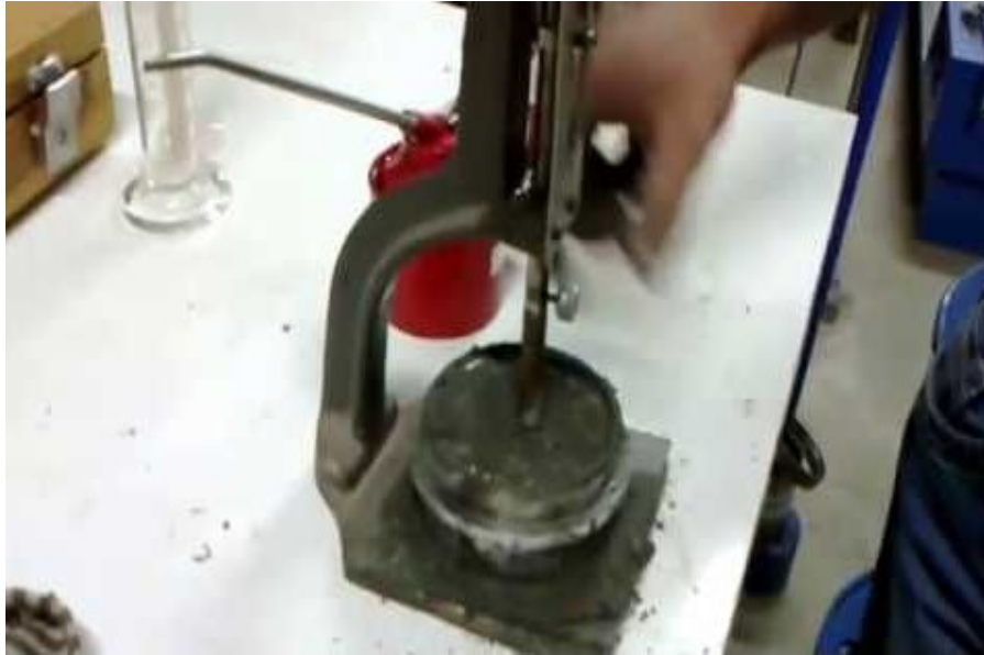
Figure 4.5 Vicat Apparatus to find Consistency and Setting time of Cement
