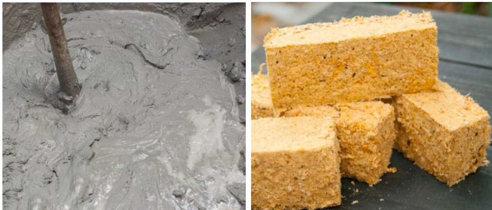
Figure 2.3 a) Stone Waste Slurry, b) Wood Saw Dust Waste Brick
