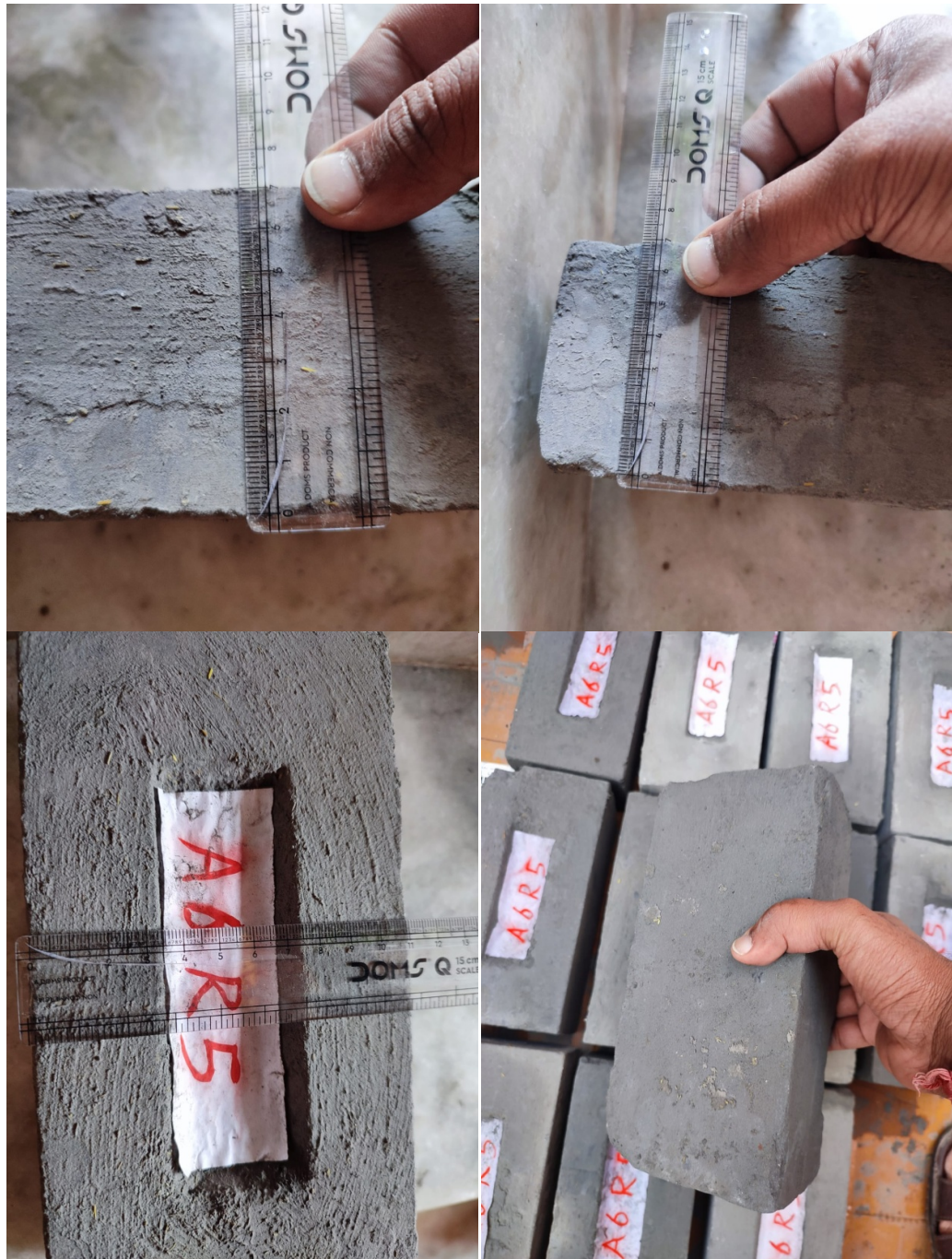
Figure 5.1 Dimensions and Tolerance (Size of Brick is 230mm x 110mm x 70mm)
