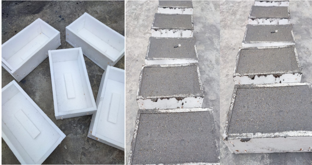
Figure 4.8 a) Required Sized Moulds, b) Filled Moulds with Mixture
