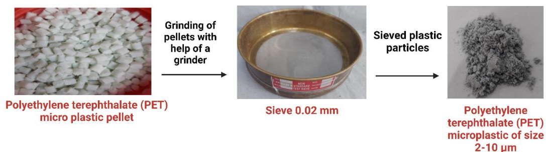
Figure 6.1: PET microplastic powder formation
