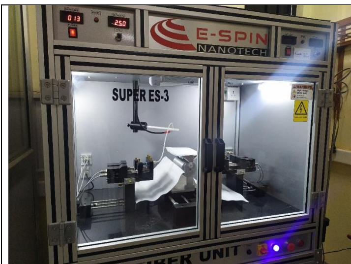
Figure 1.7. Vertical electrospinning set-up for the development of nanofibers.
