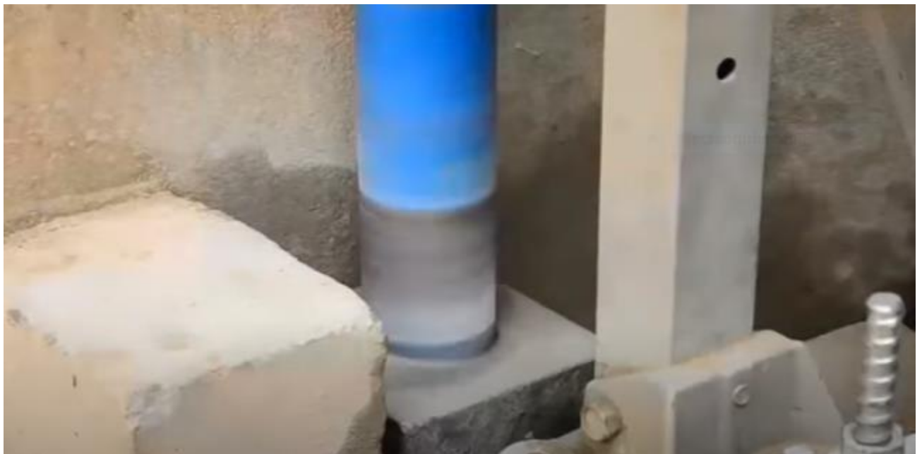
Figure 3.36 Hydraulic Drilling for Specimens
