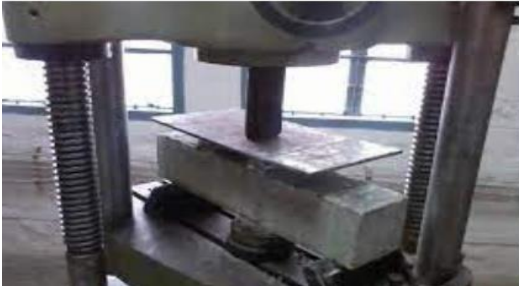
Figure 3.31 Flexural Testing Test Setup
