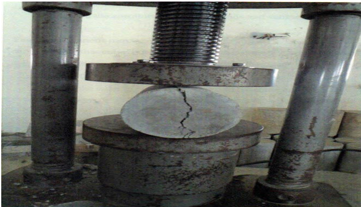
Figure 3.30 Split Tensile Test Specimen Failure
