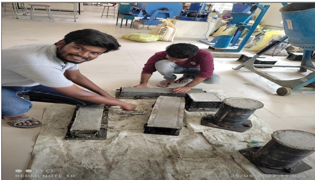
Picture 6 – Removing casted specimens from mould
