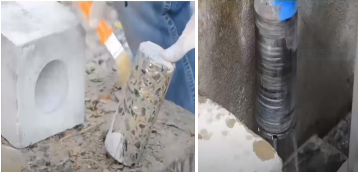
Figure 3.37 Drilled Samples for Sorptivity Test
