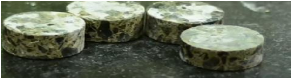
Figure 3.38 Disc Samples for RCPT Test
