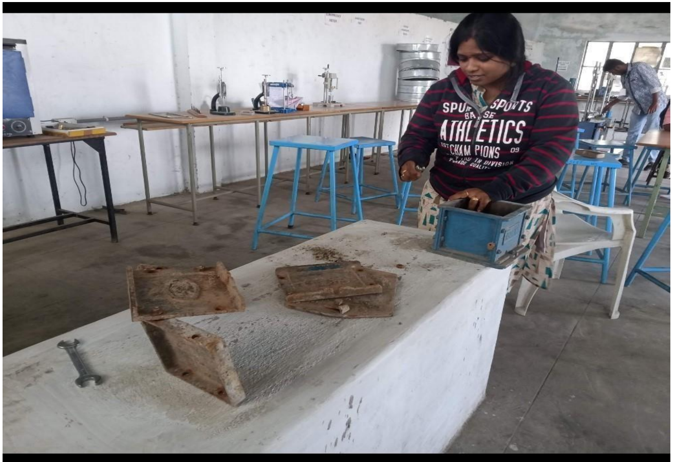
Picture 3 – Greasing Mould
