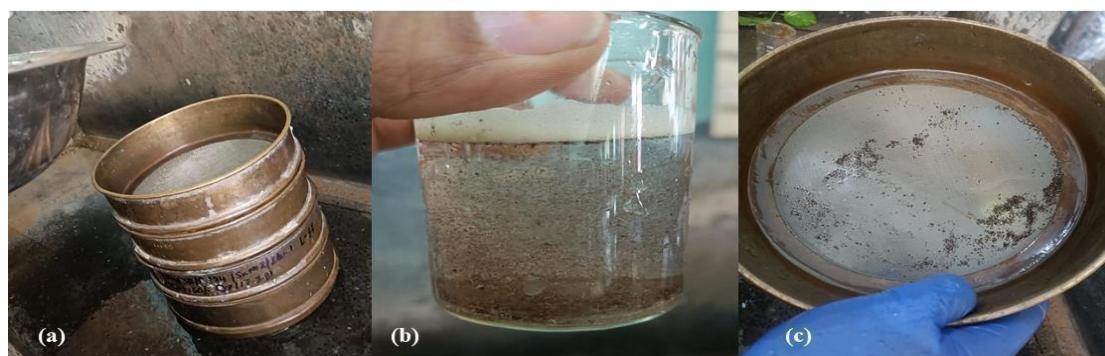
Figure 3.6 The procedure of wet-sieving and decantation; (a) emptying the upper layer of soil suspension into the sieve, (b) translucent upper layer after fine sieving, (c) fine mesh sievings
