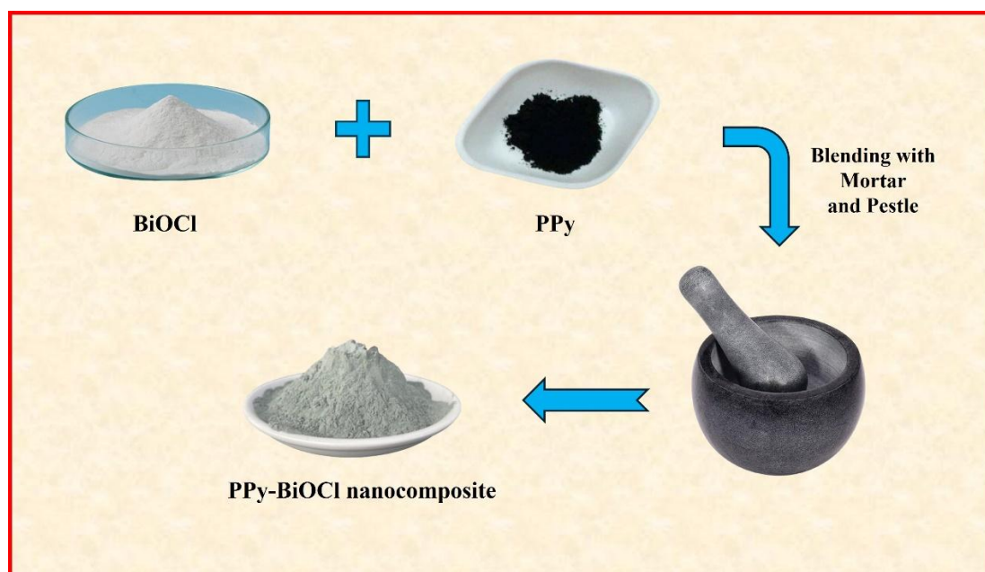
Figure 3.5. The physical blending process is employed to produce the PPy-BiOCl nanocomposites.
