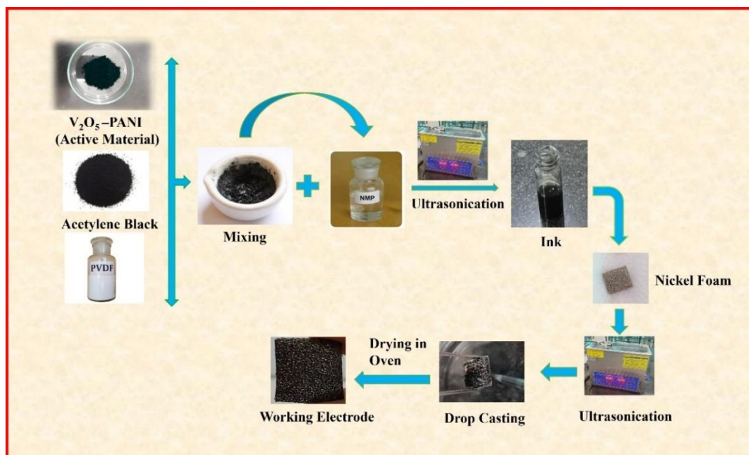
Figure 3.6. Fabrication of Supercapacitor electrodes.
