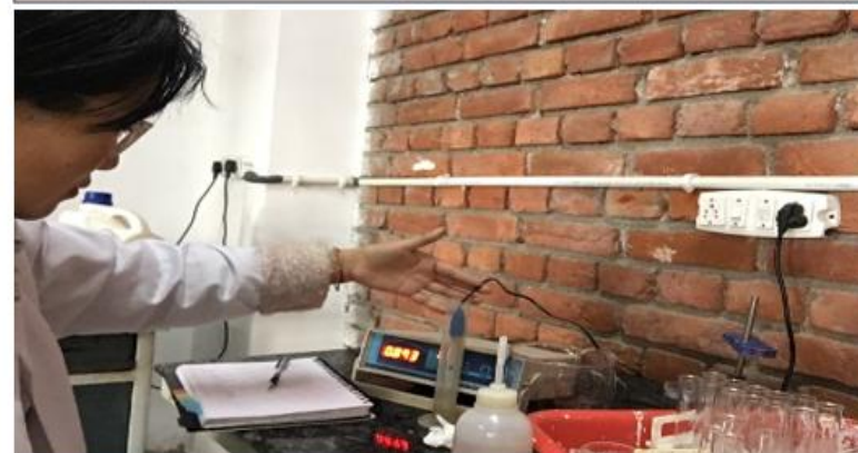
Reading of electrolytes leached out by EC meter
