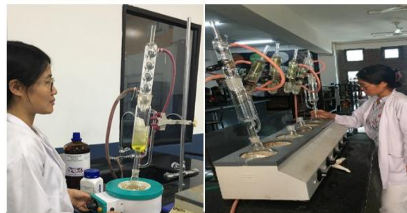
Extraction of oil by soxhlet apparatus
