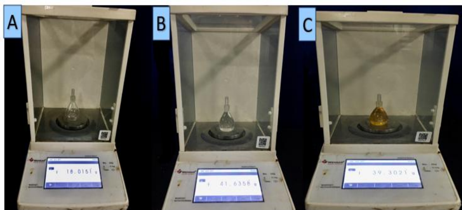
A, B, and C represents Pycnometer that is empty ,water and oil filled respectively for determining relative density of mustard oil
