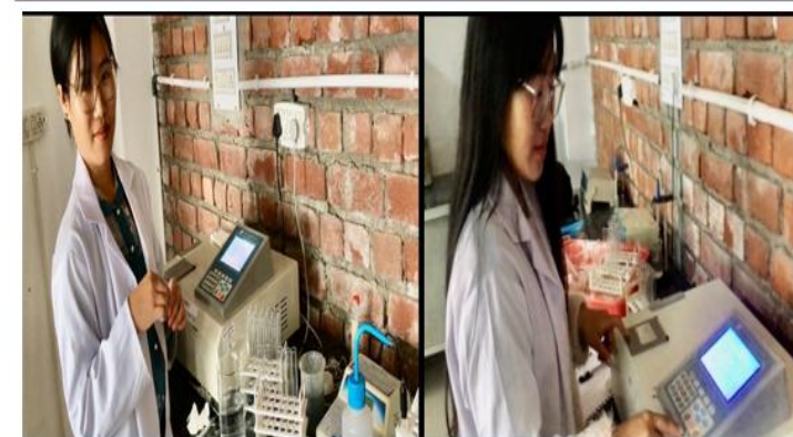
Recording optical density by spectrophotometer
