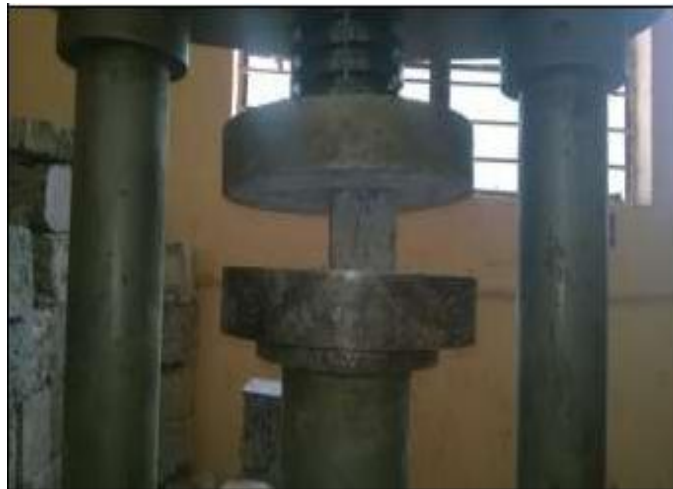
Figure. 3.4 Compressive Strength Test on Geopolymer concrete
