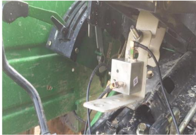
Figure 4.6 Accelerometer mounted under seat of test tractor
