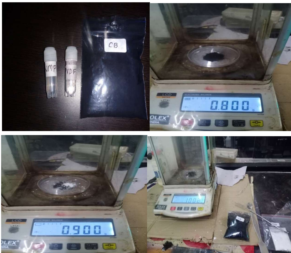
Figure 5.3: Showing 80:10:10 ratio by mass mixing of Sample with PVDF and carbon black (CB) respectively to make the final sample ready for electrode preparation.
