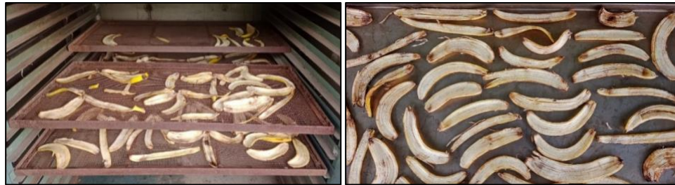
Picture 3.2: Hot air tray drying of banana peels.
