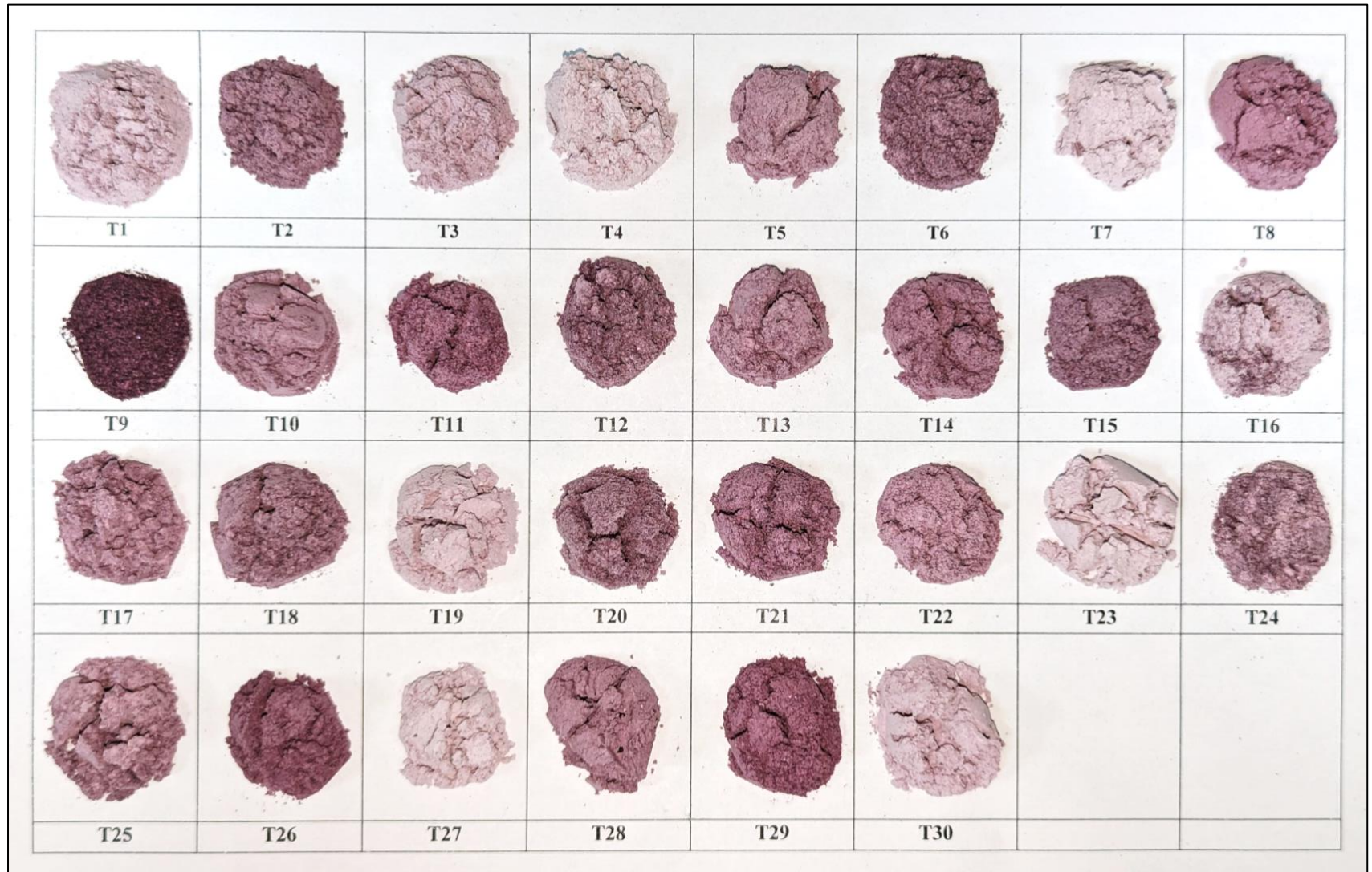
Picture 4.5: Encapsulated powder for all treatments designed by RSM-Face centred Central Composite Design
