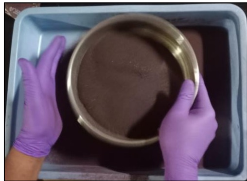
Picture 3.6: Sieving of milled powder
