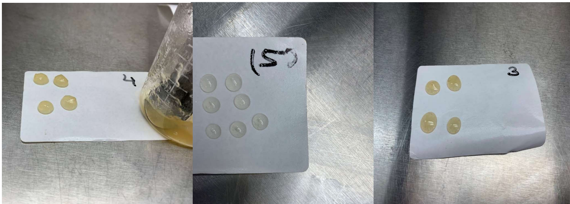
Figure 40. Pellet or disc formation using the drop method to assess different concentrations of CMC, guar gum and gelatin
