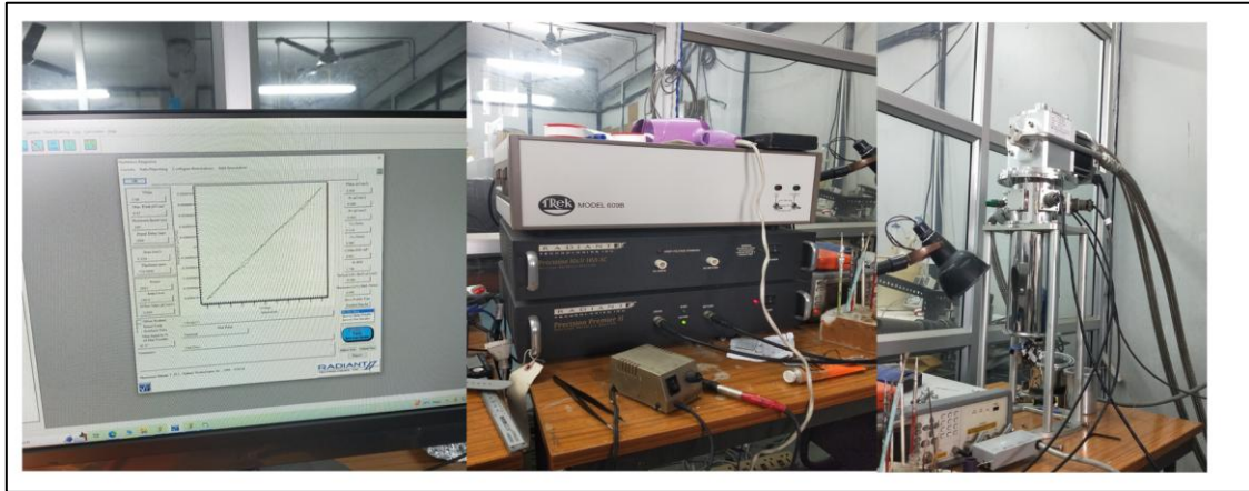
Fig.4.5 The 4 K CCR instrument setup for P-E loop measurement.
