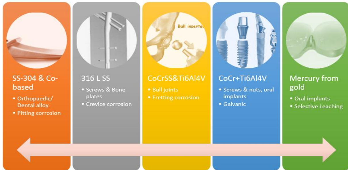
Fig 2.4. Different materials used in the various bio-medical implants in corroiосn applications .
