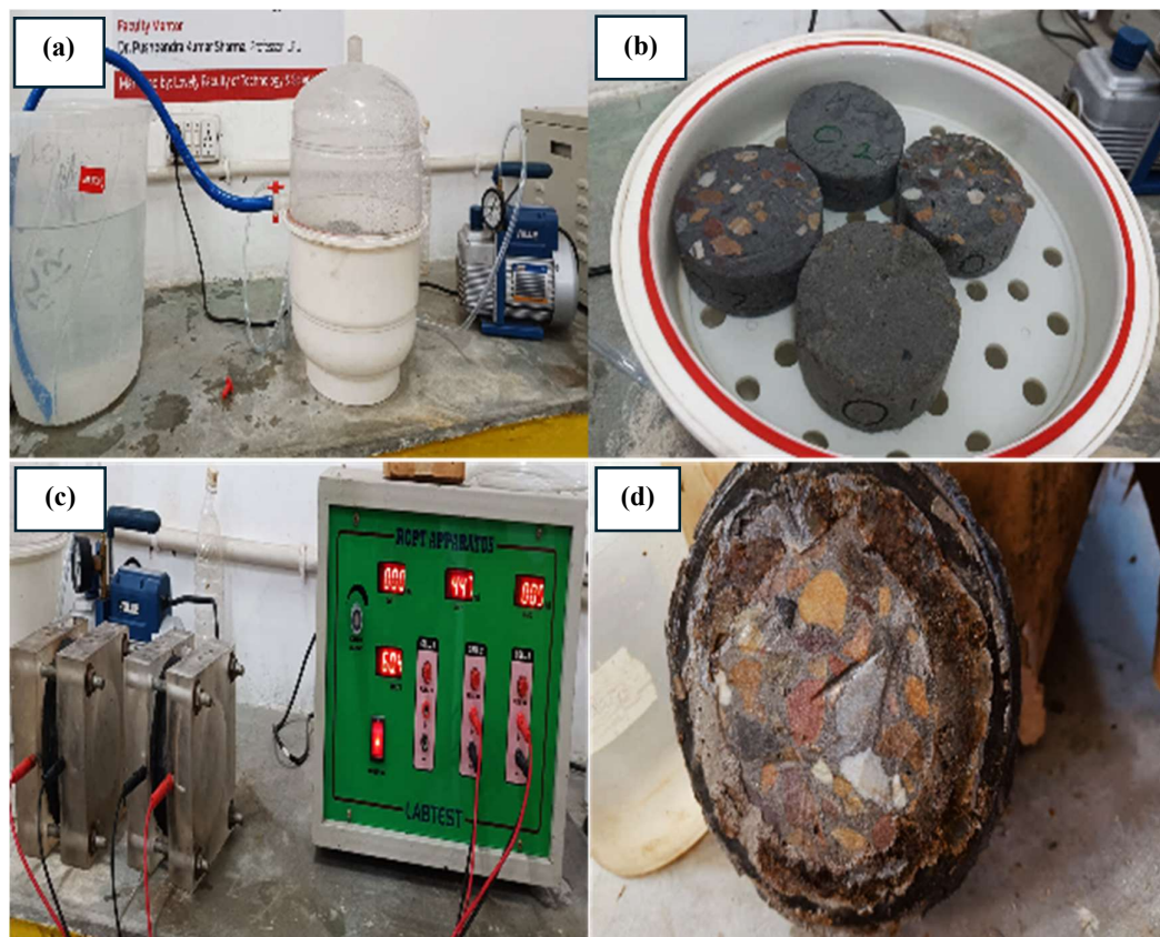
Figure 3.38 RCPT test setup (a) vacuum, (b) disc preparation, (c) apparatus and (d) after chemical penetration
