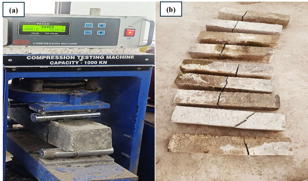
Figure 3.34 (a) FS test setup and (b) tested beam samples
