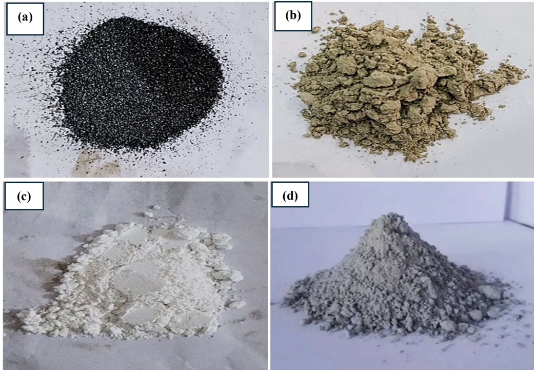
Figure 3.7 (a) IO, (b) FA, (c) LS and (d) MK used as raw materials in ferrock
