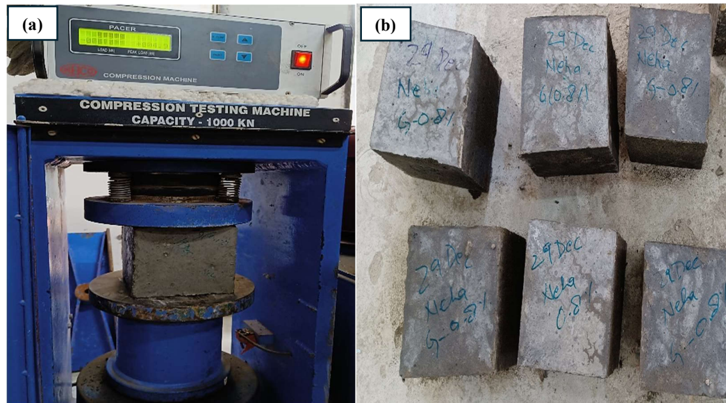
Figure 3.32 (a) CS test setup and (b) Cubes of 150 mm for testing
