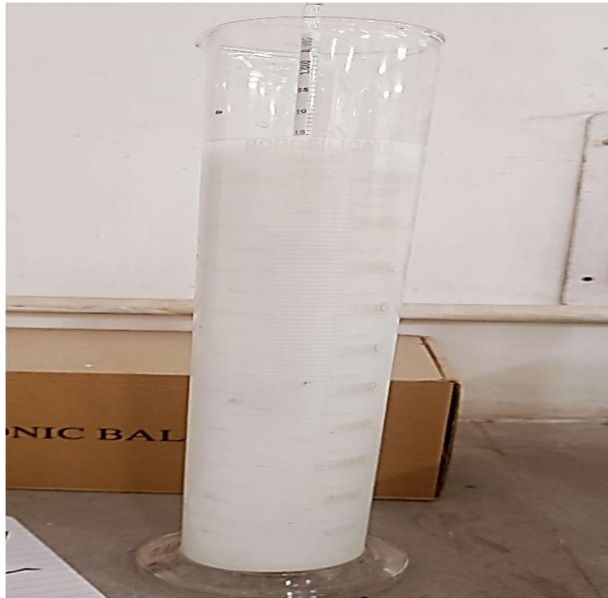
Figure 3.17 Setup of hydrograph analysis of LS
