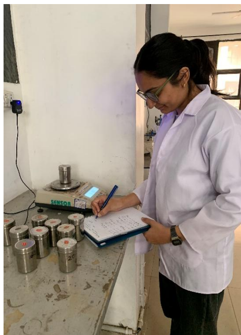
Plate 3.3: Measuring the soil moisture with the soil moisture boxes
