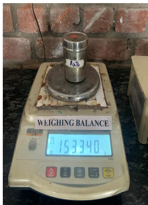
Plate 3.3: Measuring the soil moisture with the soil moisture boxes
