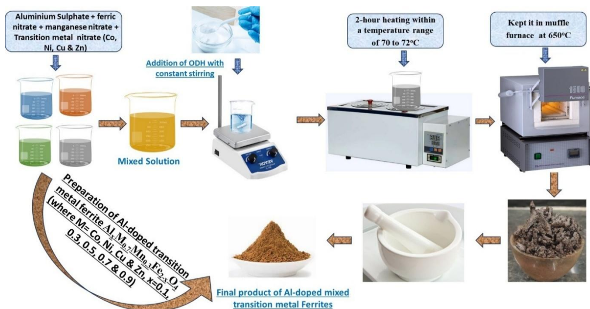
Figure 3.2: Schematic illustration of preparation of Al-doped mixed transition metal ferrite.
