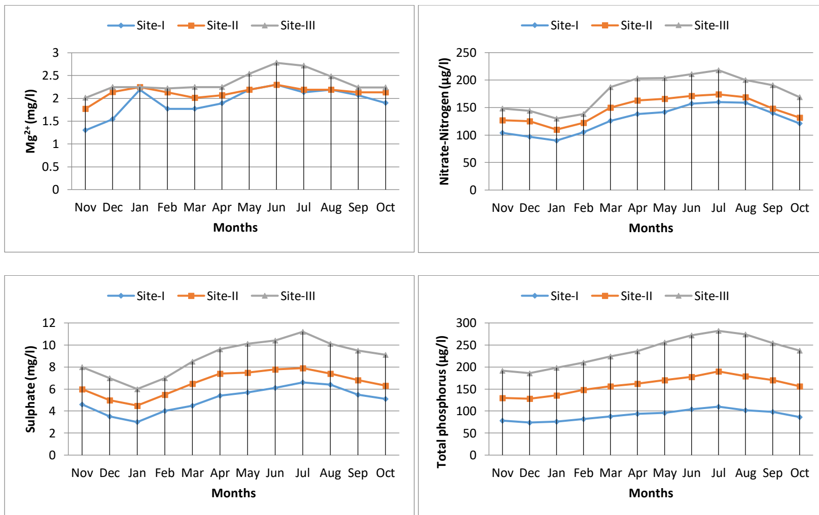
Figure 6: Showing monthly variations in Physico-chemical parameters from November, 2019 to October, 2020 at three different sites of Vaishav stream.
