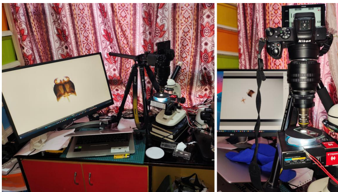
Figure 20: Micro-photography setup for slide photography
