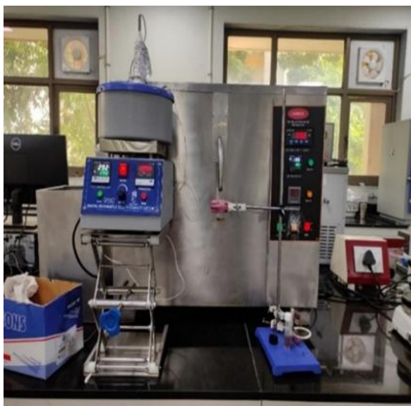
Figure 3.14 Process of bio-oil filtration through the distillation unit.
