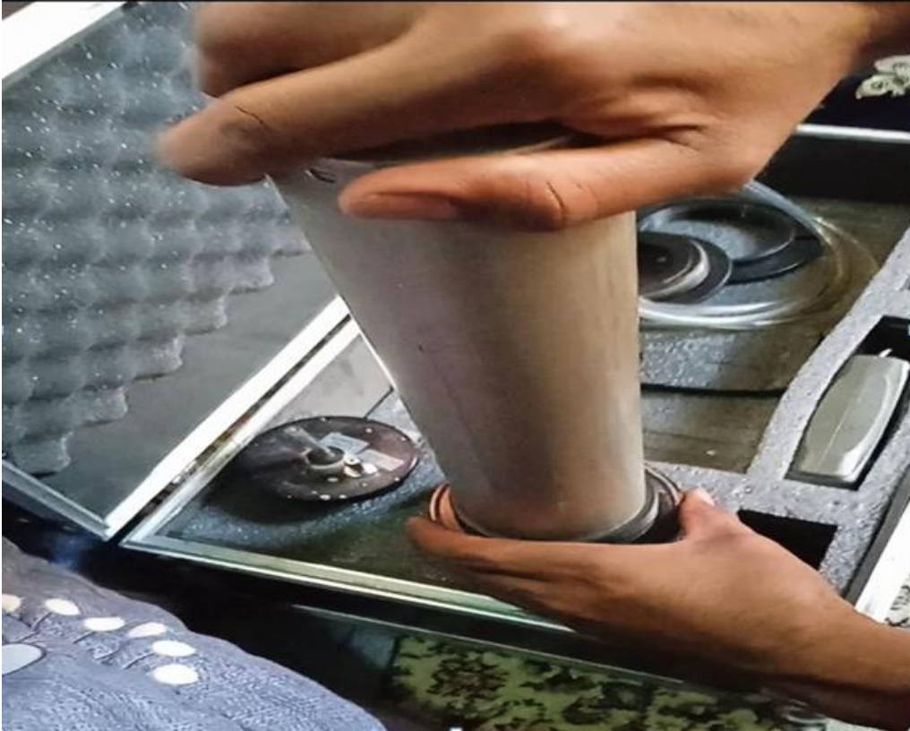
Figure 3.3: Field/ on-site estimation of the thoron flux density
