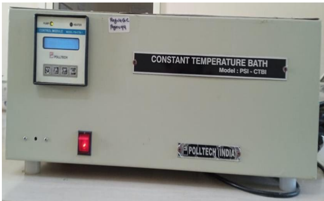
Figure 3.7: Constant temperature etching bath employed for etching of SSNTD LR-115 Detectors
