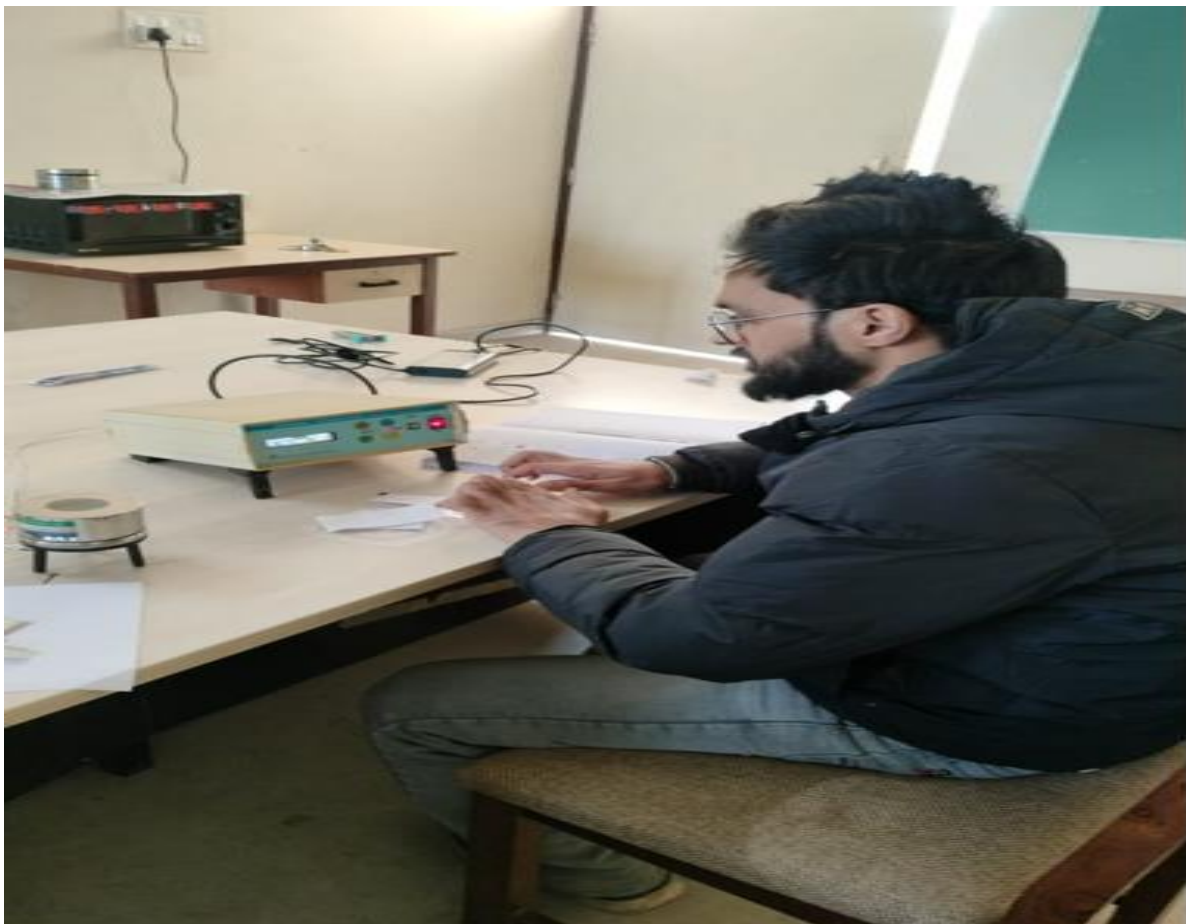
Figure 3.8: Alpha track counting analysis using a spark counter (Radiation lab Khalsa College).
