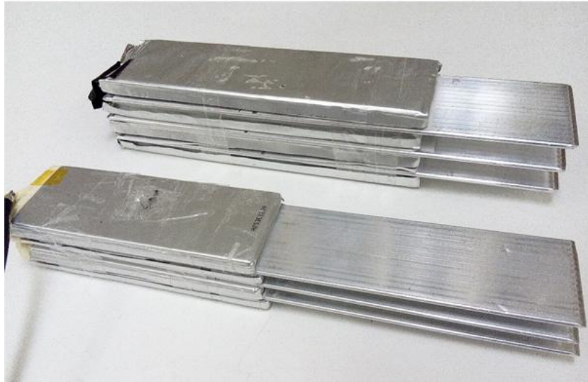
Figure 2.13: 8 Ah (top) and 3 Ah (bottom) batteries with heat pipe insertions[186]
