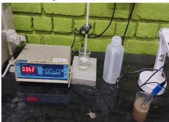
Reading data from EC meter
