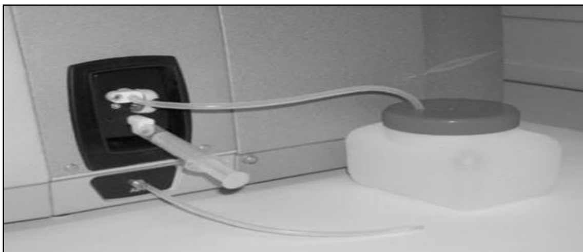
Figure 3.4: Filling of sample into sample inlet adapter
