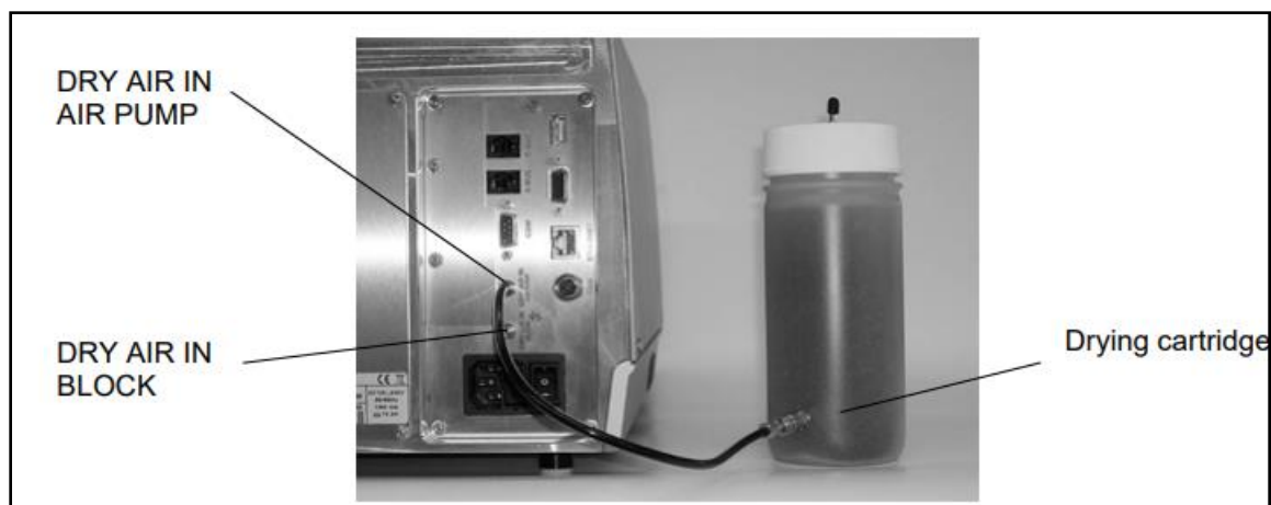
Figure 3.7: Drying cartridge connected with the instrument
