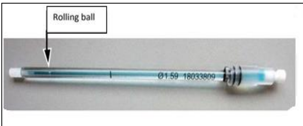
Figure 3.10: Capillary with a ball
