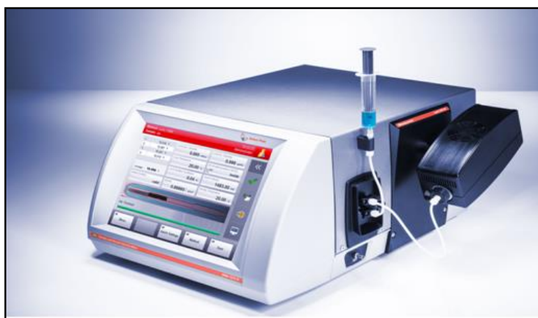
Figure 3.8: Lovis microviscometer 2000 M/ME, with DSA 5000 M
