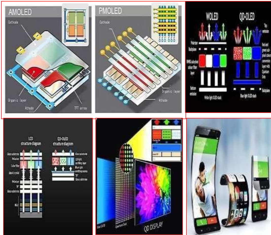
Figure 1.8: Upper row: Images of AMOLED (first left corner), PMOLED (top row middle), architectural difference between WOLED and QD -OLED (right most corner) & lower row: images of difference between QD OLED and LCD (lower left), architecture of a QD-OLED display
