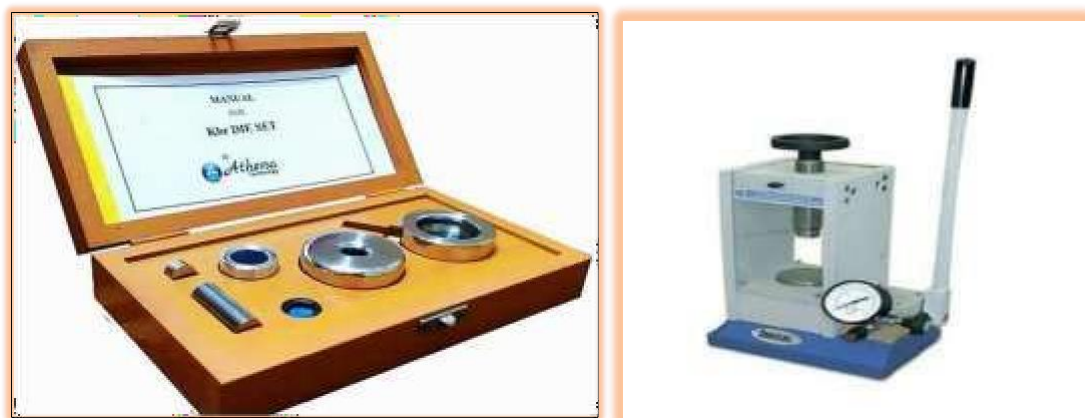
Figure 4.14.2.: Image of Athena 500x500 cold press die set box with 12 mm. diameter (left) and KBr press instrument (right)
