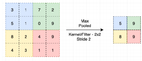
Figure 4.8 Max pooling in CNN
