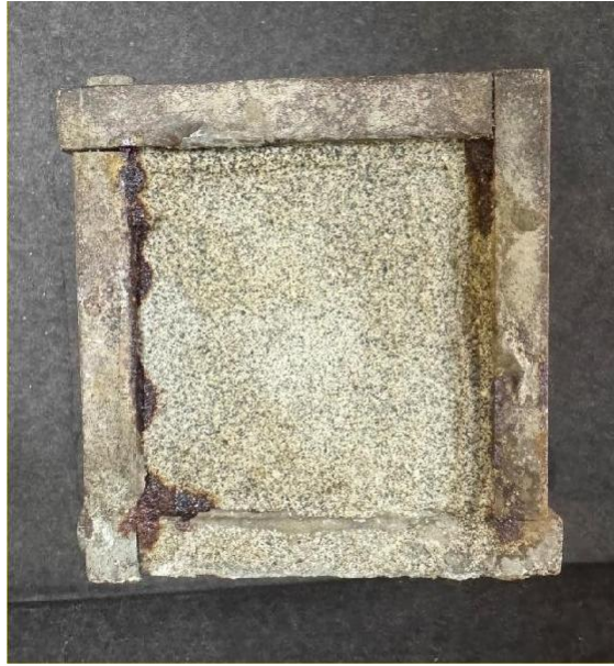
Figure 5.2: Preparation of bio-cement using cast-iron mould.
