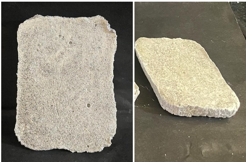
Figure 6.14: Prepared laboratory scale bio-cement bricks using fungi
