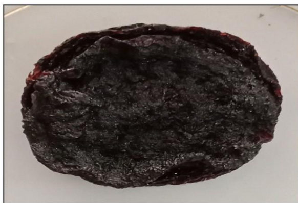
Figure 5.5: Hydrogel formed via Chemical (redox) initiation
