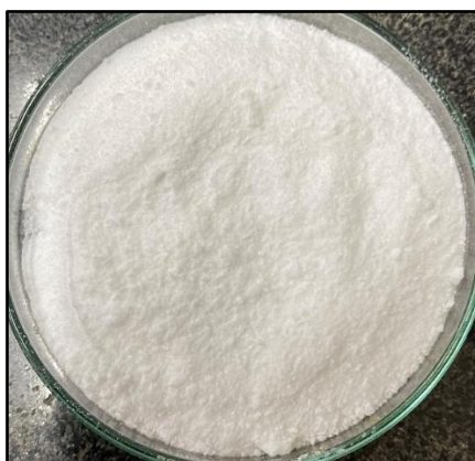
Figure 5.7: Prepared ZnO nanoparticles
