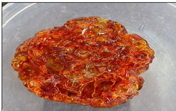
Figure 5.1: Synthesized BM-g-poly(AA) hydrogel
