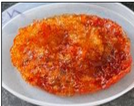
Figure 5.4: Hydrogel formed via Thermal polymerization
