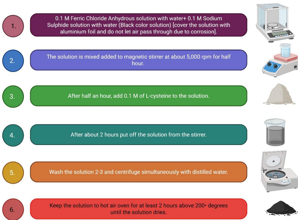
Figure 3.2: Methodology of the synthesis of Iron Sulphide Quantum dots
