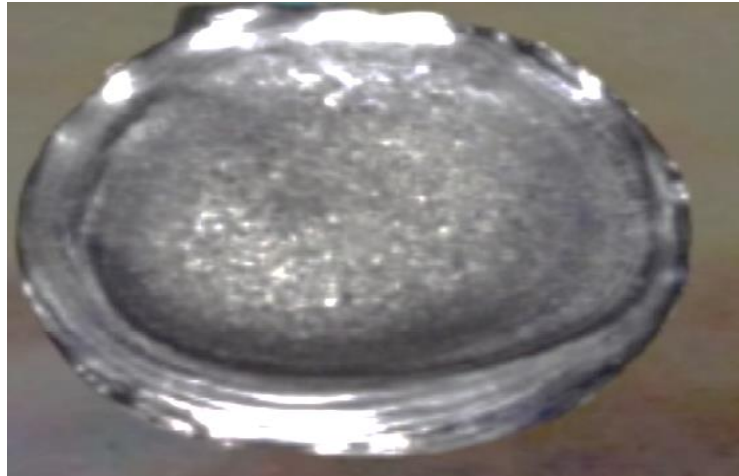
Figure 4.5 As cast \beta -phase Ti alloy by vacuum arc melting Process
