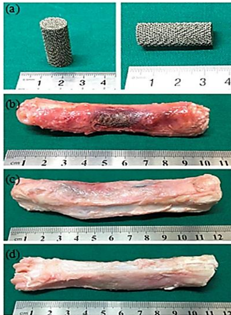
Figure 2.8 In vivo study of implantation on porous Ti alloy implant (Singh et al., 2022)
