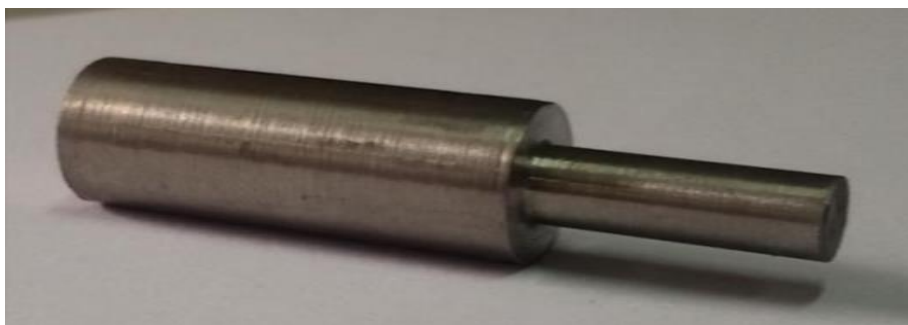
Figure 4.7 Shape and size of tool electrode.
