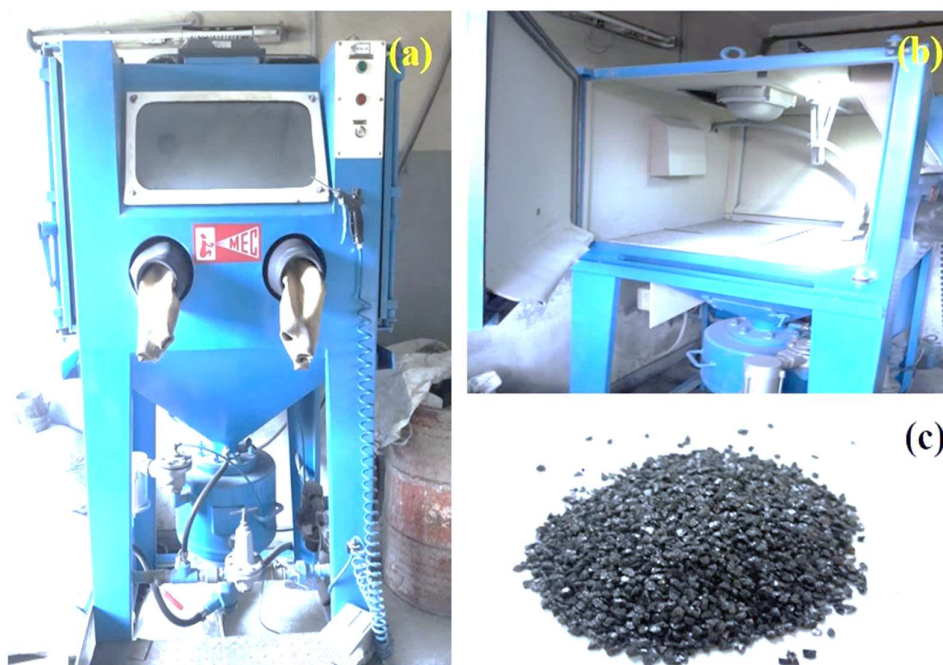
Fig.3.1. (a) Front and (b) side view of shot blasting machine and, (c) Blasting medium (Virgin alumina).
