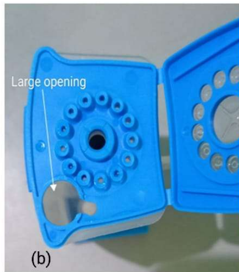
Figure 25- (a) disposable sterile pipette and (b) cartridge showing large opening for sample
