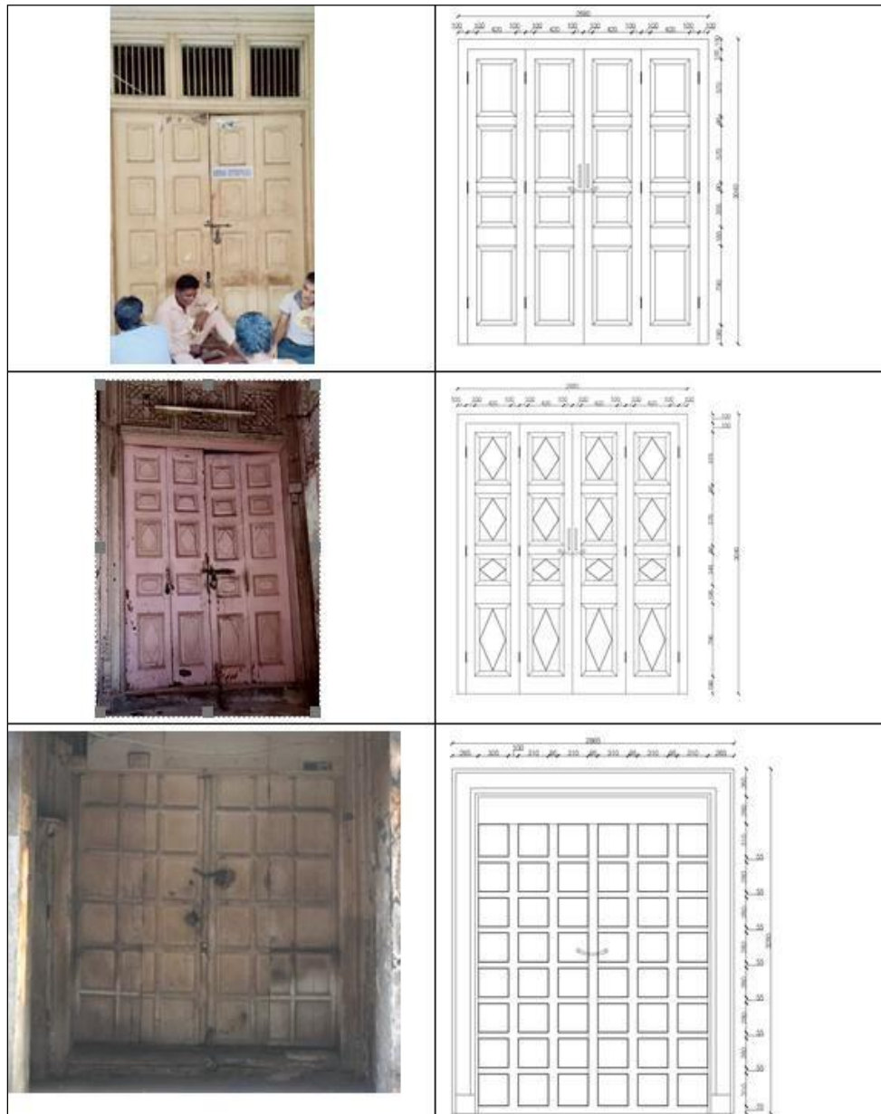
Figure 5.8: Documentation Drawing of Traditional Wooden Doors, Katra Ahluwalia.
