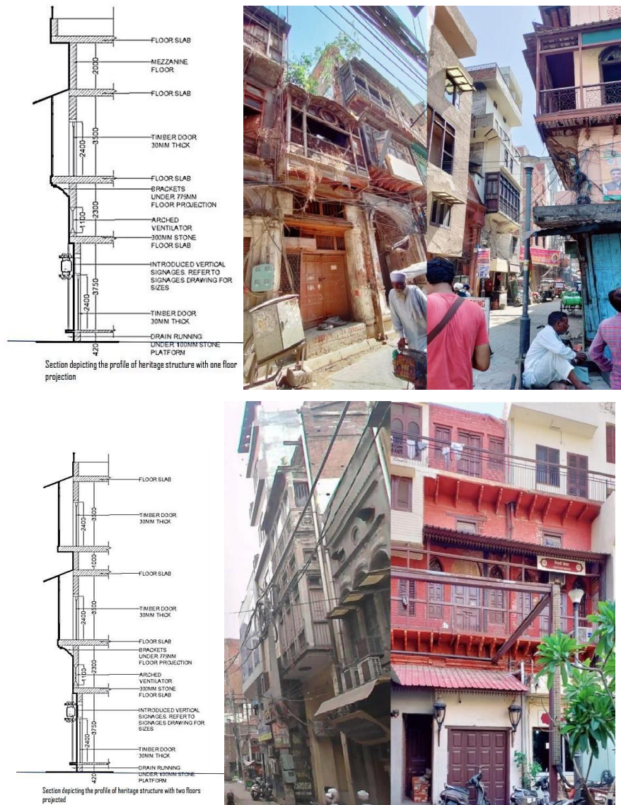
Figure 5.26: Sectional outer profile of historic buildings
