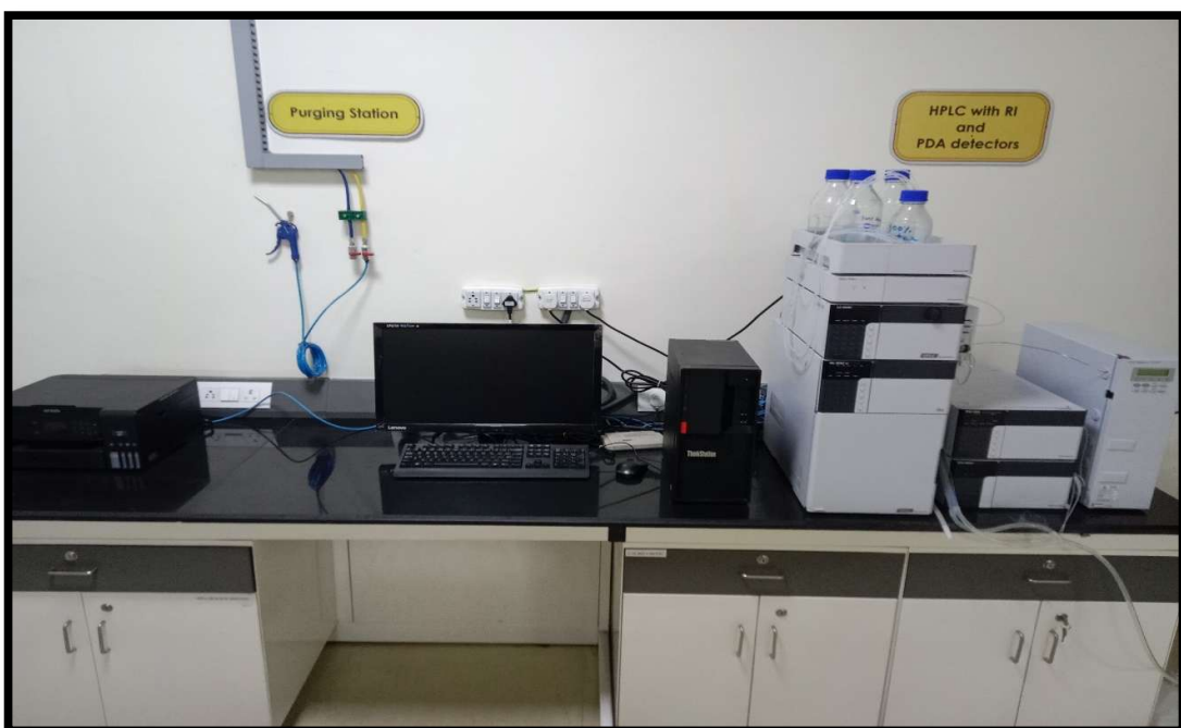
Plate 15. Estimation of different treatments residues in brinjal fruits using HPLC with RI and PDA detectors
