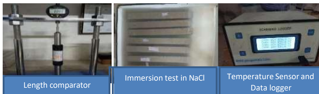
Fig. 5.8 Arrangements for Durability test of concrete
