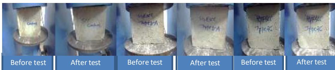
Fig.5.27 Compressive strength test of SCC Control ,Hy FSCC-Type1 and Hy FSCC-Type2 recipes
