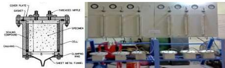
Fig.5.23 Permeability test arrangements as per IS 516(Part 2/Sec1):2018
