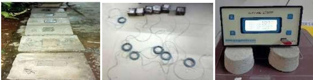
Fig.6.14 SCC HyFR-NA1.5 panels and casted specimens placed by the side of study area to observe distress and maturity
