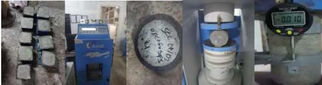
Fig.5.10 Compression testing and Tensile Splitting Strength testing and MoE test of SCC FMKseries and SCC GMKseries specimens
