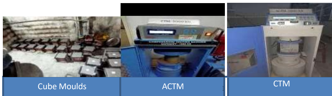
Fig. 5.7 Arrangements for mechanical testing of concrete
