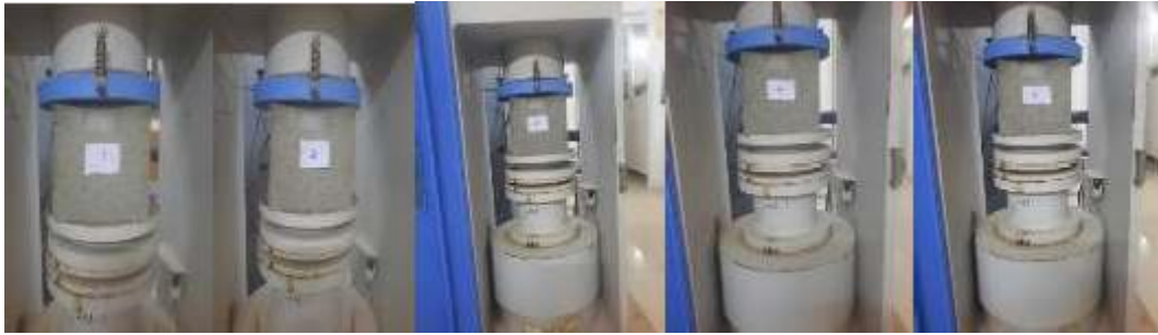
Fig.5.33 Failure pattern under compression of SCC HyFR-NA0.00 and SCC HyFR-NA mix at 28-days
