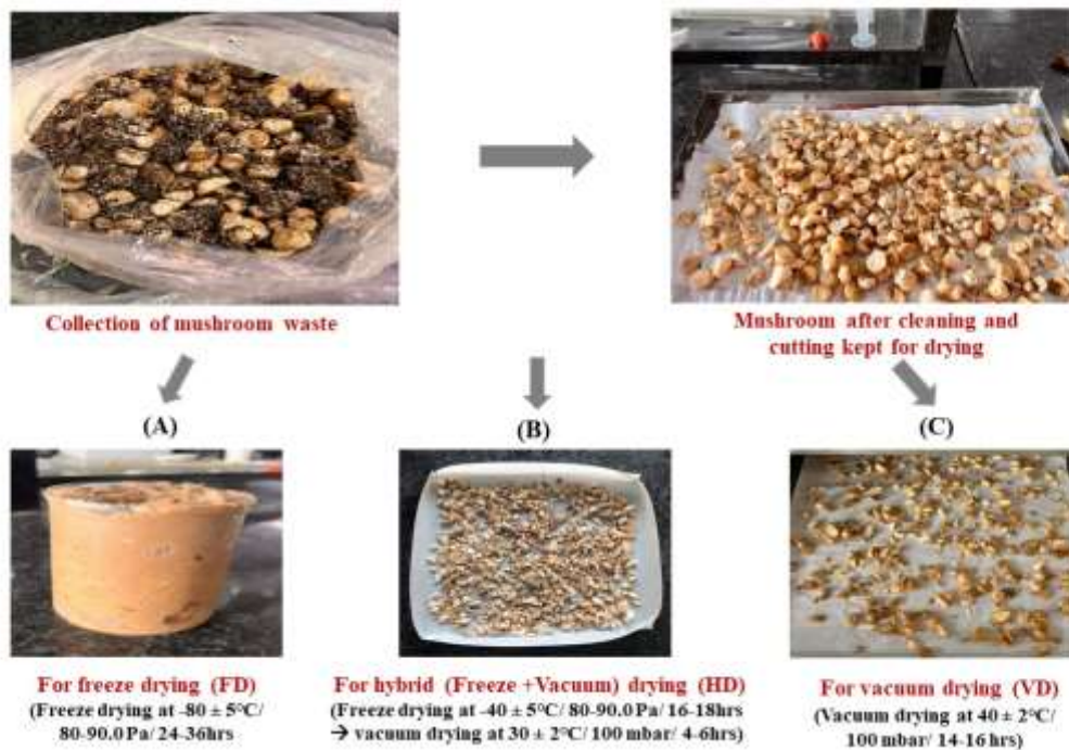
Figure 4.2. Pictorial representation of production of mushroom waste powder (MWP) using different drying methods.
