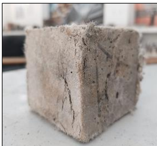
Figure 37: Cracks on ECC cube after Compression Test
