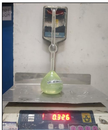
Figure 20: Specific Gravity Test of Fly Ash
