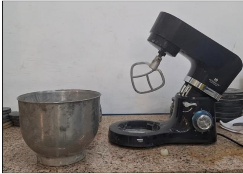
Figure 26: Mixer with planetary rotating blade
