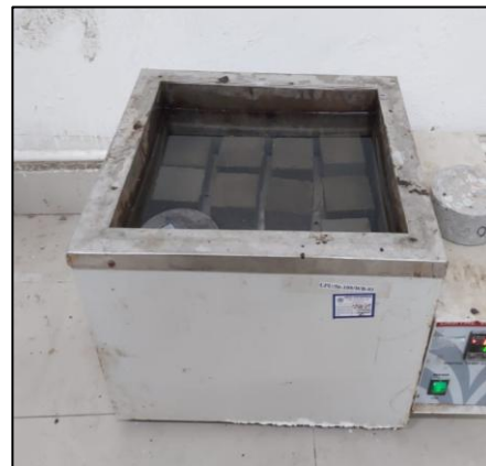
Figure 35: Curing of ECC Cubes
