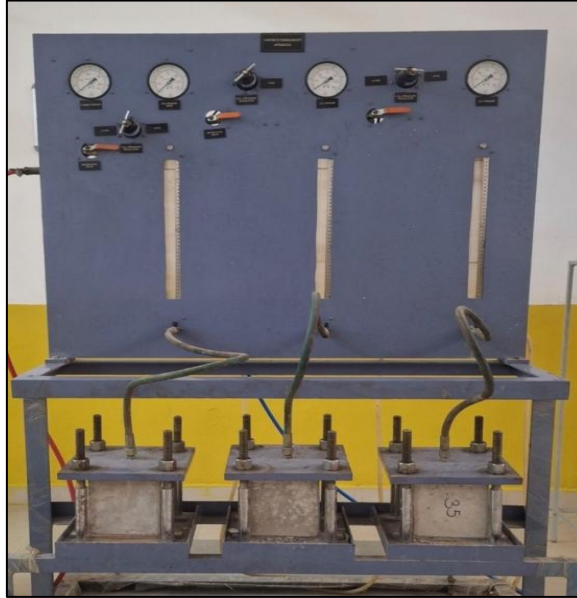
Figure 48: Water Permeability Test Set-up
