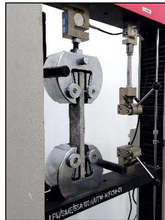
Figure 40: Direct Tensile Testing Set-up
