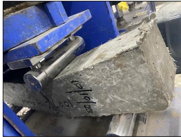
Figure 44: Flexural Test Set-up
