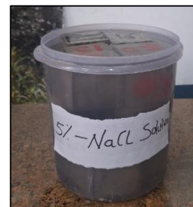
Figure 50: ECC specimen in the solution of 5% NaCl
