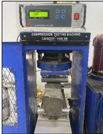
Figure 43: Flexural Test Set-up
