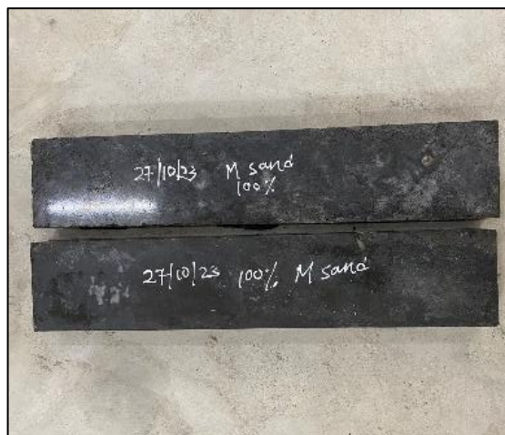
Figure 42: ECC casted Beam Specimens
