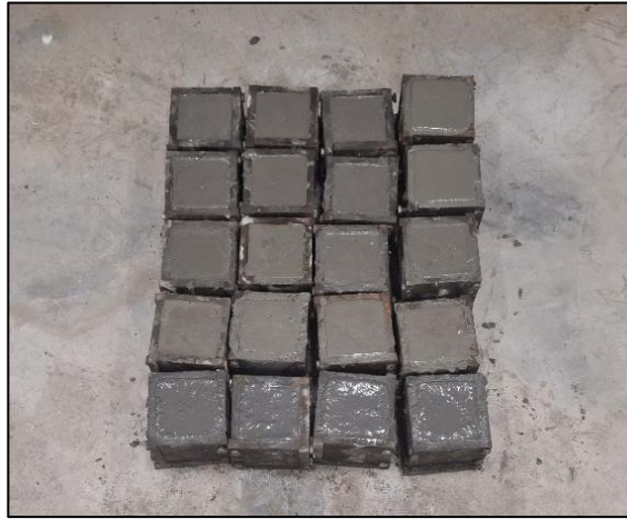
Figure 27: Freshly casted ECC cubes
