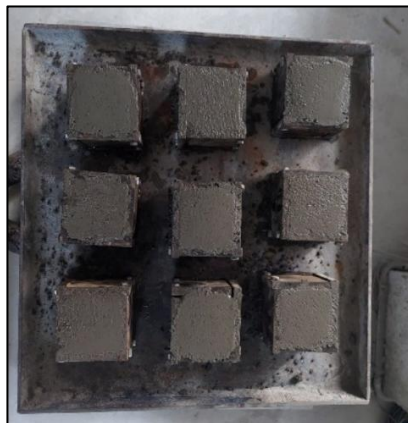
Figure 34: Casting of ECC Cubes
