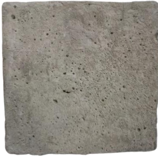
Figure 53: ECC Cube before Chloride Attack
