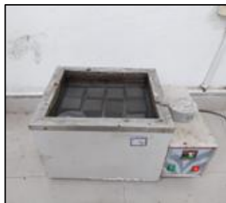
(e) Curing of the Cement Mortar Specimens in water bath
