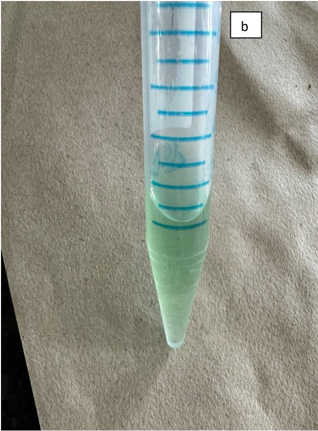
P 4.3: (a) Ash content of tubers; (b) Anthrone reagent method used for the analysis of starch content of tubers
