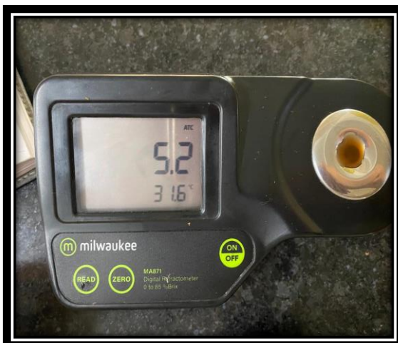
Plate 3.14: Measuring TSS with refractometer
