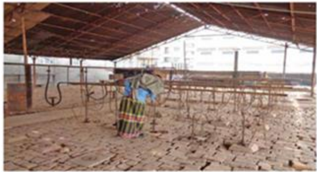
Figure 1.11: Use of natural gas in a Hoffman kiln in Bangladesh.
