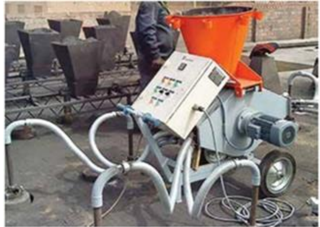
Figure 1.13: Trickle feeder for feeding biomass fuel in kiln.
