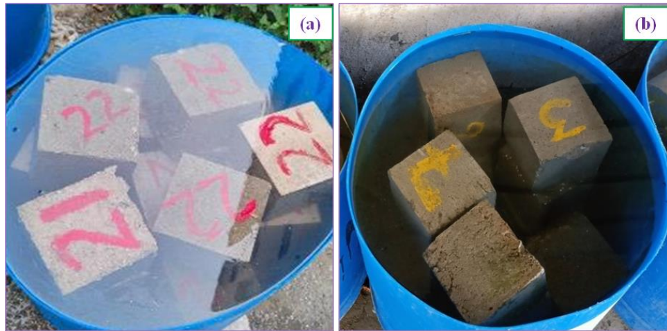
Fig: 3.11 (a) Cubes immersed in water. (b) Cubes immersed in HCL solution.
