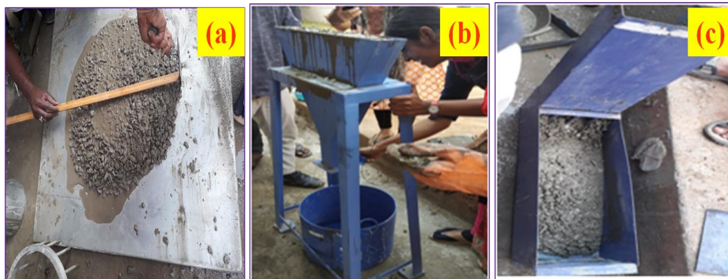
Fig.3.9: Fresh property tests (a) Slump flow (b) V Funnel (c) L –Box
