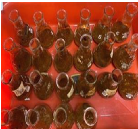
Fig.11 and 12: Digestion of seed and straw sample in hot plate.
