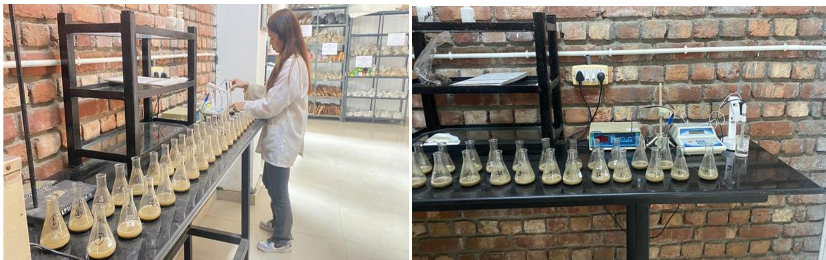
Fig.25 and 26: Estimation of soil EC using EC meter.
