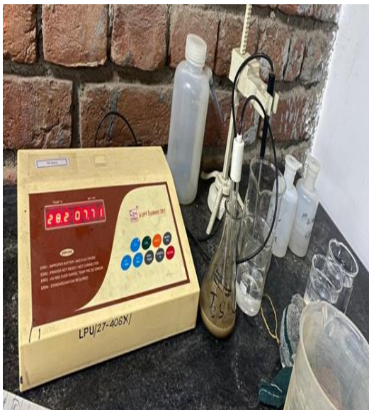
Fig. 27 and 28: Estimation of soil pH using PH meter.
