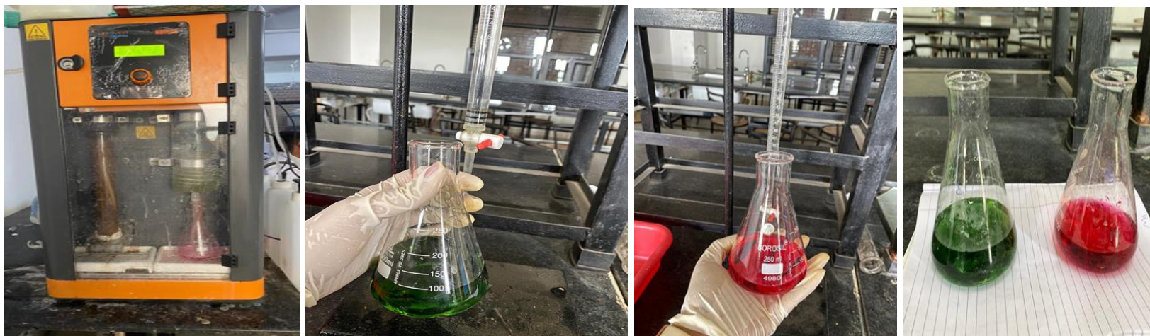
Fig.42: Distillation and titration of soil sample for estimation of available nitrogen.
