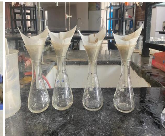
Fig.32: Filtration of soil after mechanical shaking.
