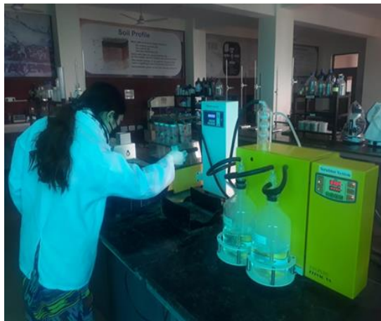
Fig.6 and 7: Digestion of grain and straw sample for estimation of total nitrogen
