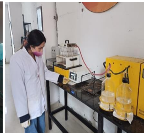
Fig.6 and 7: Digestion of grain and straw sample for estimation of total nitrogen
