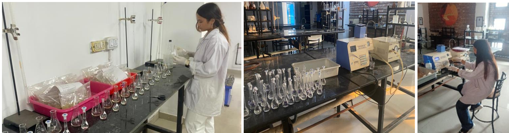
Fig.33, 34 and 35: Preparation and analysis of soil sample for estimation of available potassium using Flame photometer.
