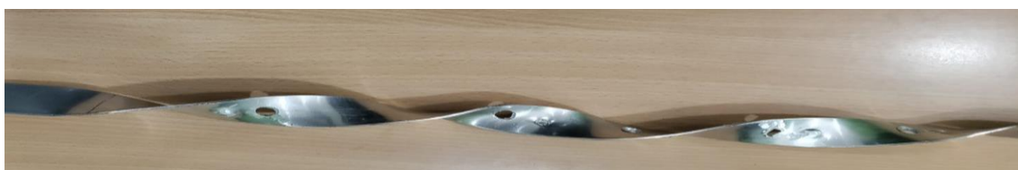
Fig.3.25 Photograph of twisted tape with dimples (D =2mm D/H=1.5)
