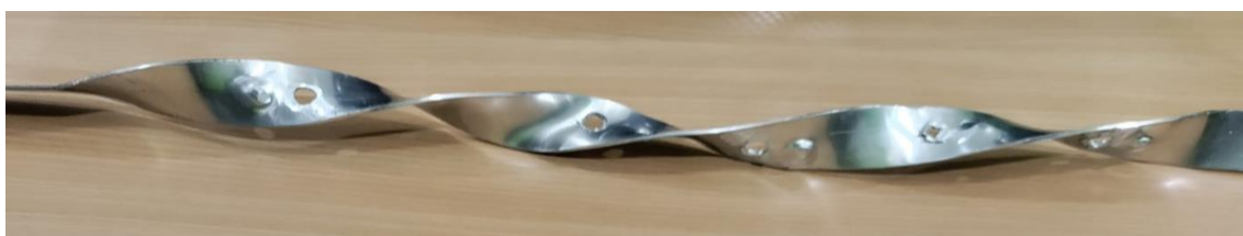
Fig. 3.24 Photograph of twisted tape with dimples (D =2 mm D/H=3)
