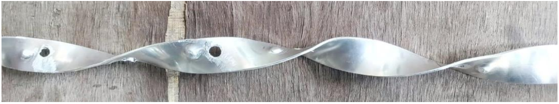
Fig. 3.26 Photograph of twisted tape with dimples ( D =4 \text{ mm } D/H=4.5 )
