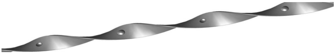
Fig. 3.4 Wire frame model of double pipe heat exchanger with dimpled twisted tape
