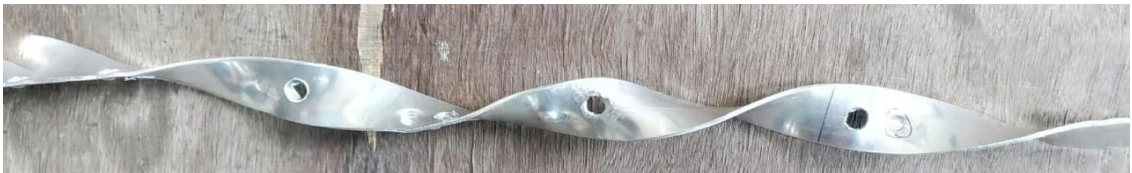
Fig. 3.27 Photograph of twisted tape with dimples ( D =4 \text{ mm } D/H=3 )
