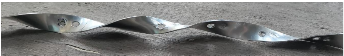
Fig.3.31 Photograph of twisted tape with dimples ( D =6 \text{ mm } D/H=1.5 )
