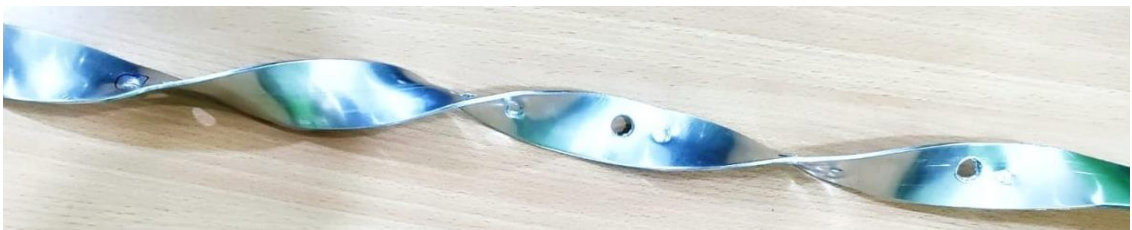
Fig.3.30 Photograph of twisted tape with dimples ( D =6 \text{ mm } D/H=3 )
