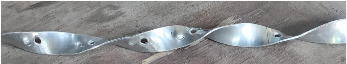
Fig.3.29 Photograph of twisted tape with dimples ( D =6 \text{ mm } D/H=4.5 )
