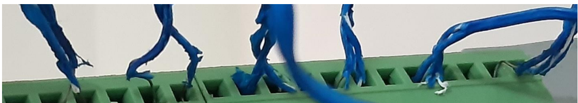
Fig.3.9 Photograph of T-type thermocouples used in experiment
