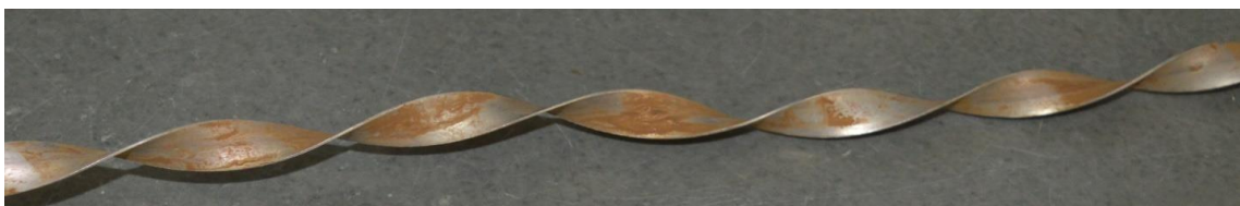
Fig.3.22 Photograph of Plain twisted tape
