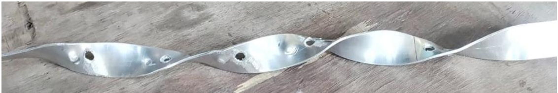
Fig. 3.28 Photograph of twisted tape with dimples ( D =4 \text{ mm } D/H=1.5 )
