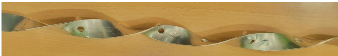
Fig. 3.23 Photograph of twisted tape with dimples (D =2 mm D/H=4.5)
