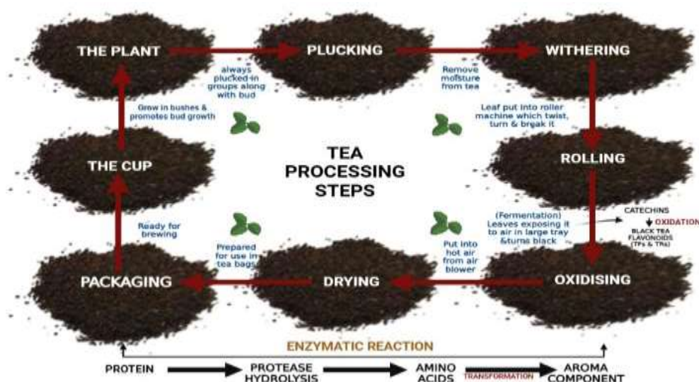
Fig. 18: Pictorial representation of different steps involved in manufacturing of Tea (created in www.Biorender.com )
